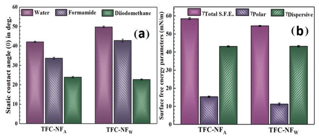
Hydrophilic characters (a) and surface free energy parameters (b) of TFC-NF membranes, TFC-NF<sub>A</sub> and TFC-NF<sub>W</sub>.
