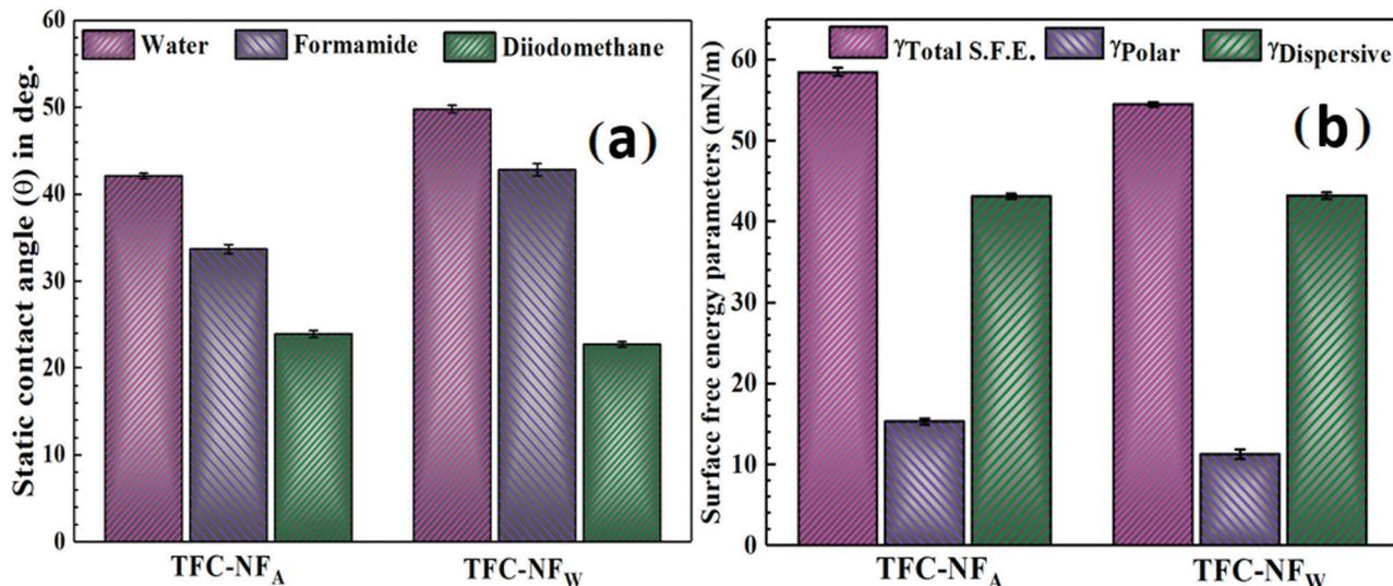
Fig. 6 Hydrophilic characters (a) and surface free energy parameters (b) of TFC-NF membranes, TFC-NF<sub>A</sub> and TFC-NF<sub>W</sub>.
