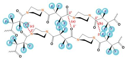
Fig. 3 Structural representation of the skin layer polymer FPA, highlighted with the possible attenuated secondary non-covalent type interactions (a and b) and charge-transfer complex formation (c).
