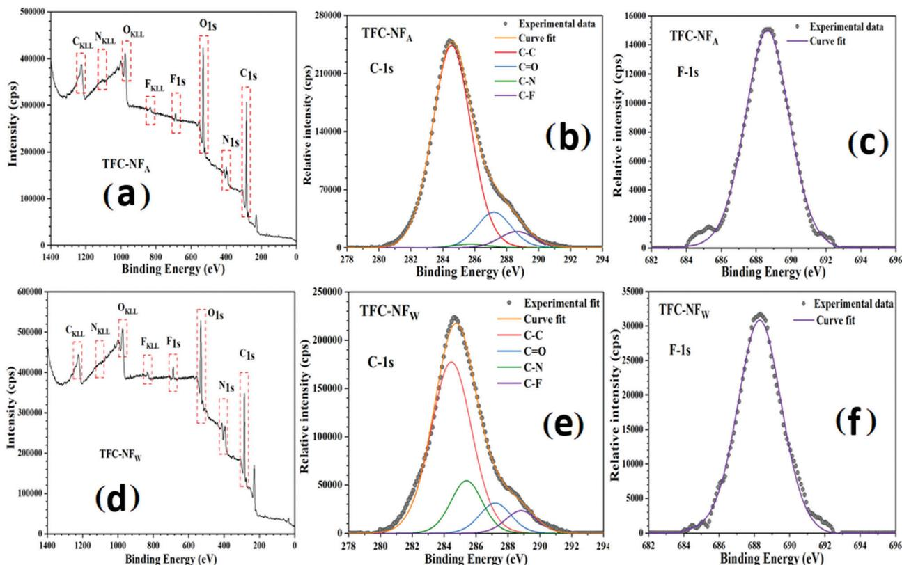
Fig. 2 XPS survey scan spectra (a and d); and high-resolution TFC-NFs (b and e) and F-1s (c and f) spectra of membrane skin layers for TFC-NF<sub>A</sub> and TFC-NF<sub>W</sub>, respectively.
