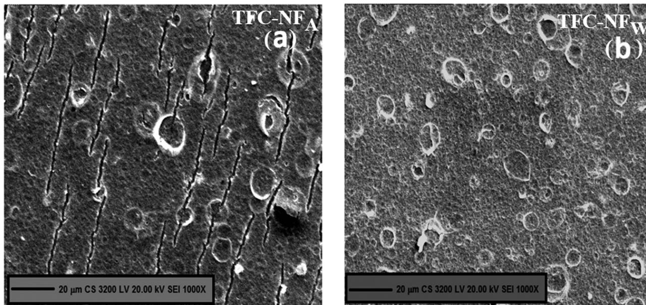
Fig. 5 Skin surface morphology of FPA-based TFC-NF membranes, (a) TFC-NF<sub>A</sub> and (b) TFC-NF<sub>W</sub>, prepared by exposing them to two different environments during fabrication.
