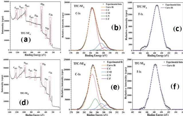
Fig. 2 XPS survey scan spectra (a and d); and high-resolution C-1s (b and e) and F-1s (c and f) spectra of membrane skin layers for TFC-NFA and TFC-NF<sub>w</sub>, respectively.
