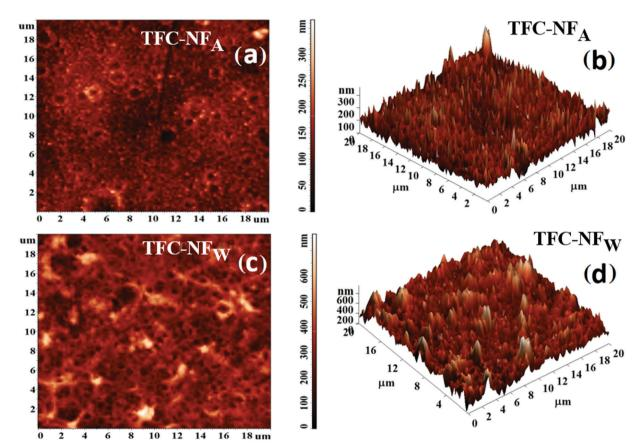
Fig. 4 Skin surface topographies of FPA-based TFC-NF membranes, prepared by exposing them to two different environments during fabrication: (a and b) 2D and 3D AFM images of TFC-NF<sub>A</sub> and (c and d) 2D and 3D AFM images of TFC-NF<sub>W</sub>.
