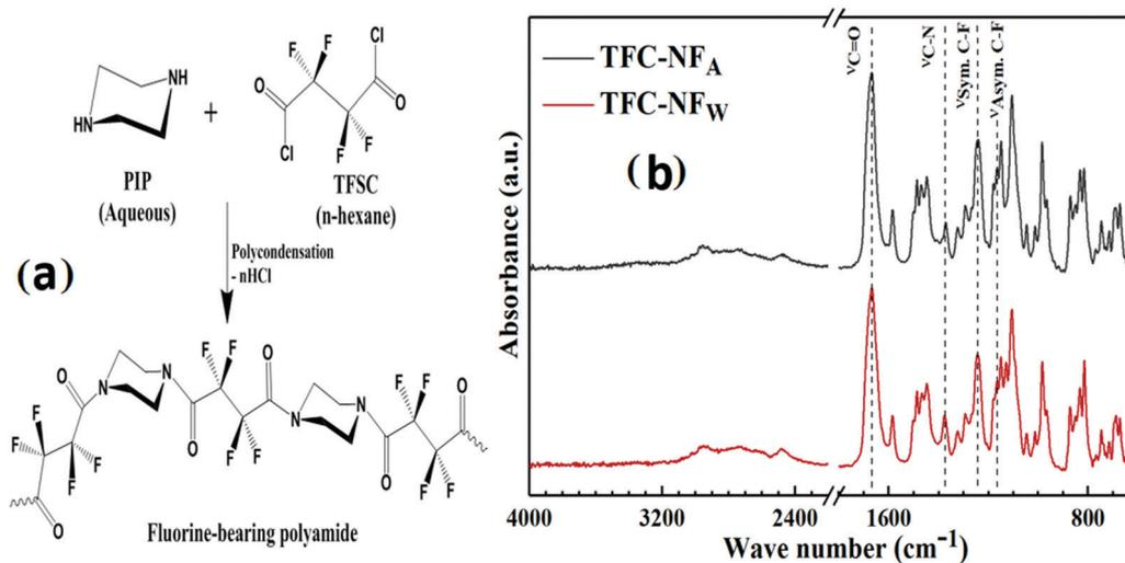
Fig. 1 (a) Reaction scheme for *in situ* interfacial polymerization between PIP, as a diamine monomer, and TFSC, as a fluorine-bearing diacyl chloride monomer, to derive the skin layer polymer FPA of TFC-NF membranes; and (b) ATR-FTIR spectra of TFC-NF<sub>A</sub> and TFC-NF<sub>W</sub> over 600–4000 cm<sup>-1</sup>.
