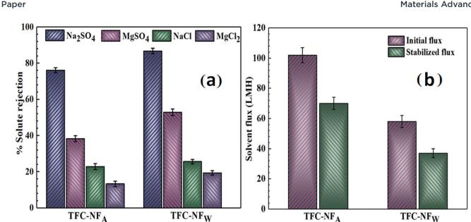
Fig. 7 Nanofiltration performances of TFC-NF membranes: (a) solute rejection against isosmotic solutions of NaCl, Na<sub>2</sub>SO<sub>4</sub>, MgCl<sub>2</sub> and MgSO<sub>4</sub>; and (b) initial and stabilized solvent fluxes of the membranes.
