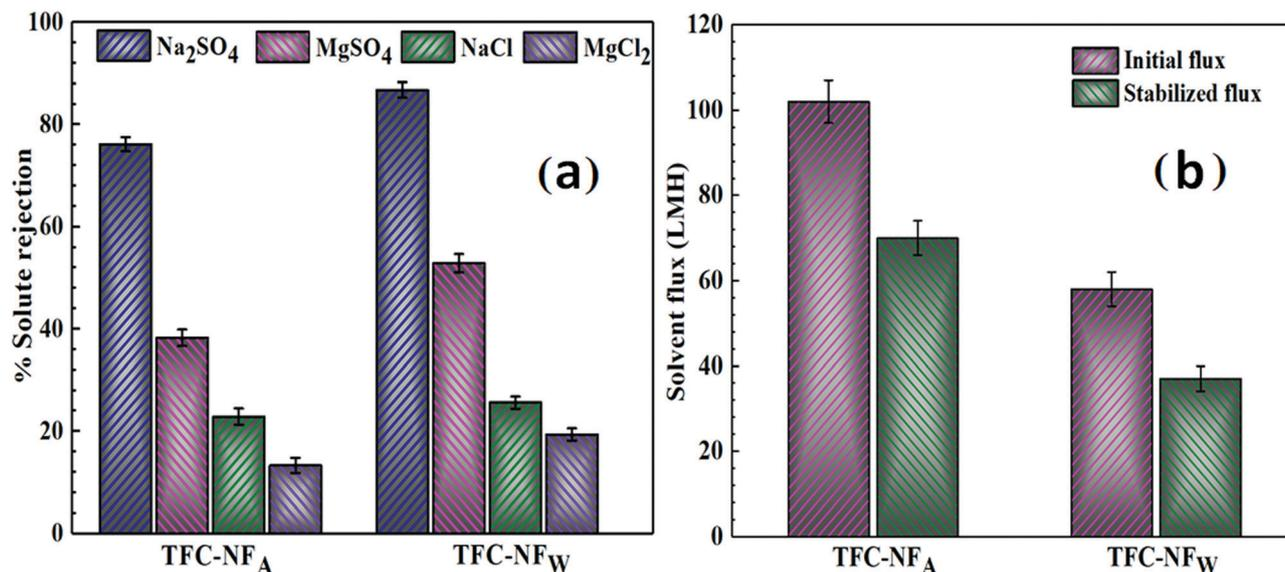
Fig. 7 Nanofiltration performances of TFC-NF membranes: (a) solute rejection against isosmotic solutions of NaCl, Na<sub>2</sub>SO<sub>4</sub>, MgCl<sub>2</sub> and MgSO<sub>4</sub>; and (b) initial and stabilized solvent fluxes of the membranes.
