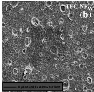
Fig. 5 Skin surface morphology of FPA-based TFC-NF membranes, (a) TFC-NF<sub>A</sub> and (b) TFC-NF<sub>W</sub>, prepared by exposing them to two different environments during fabrication.
