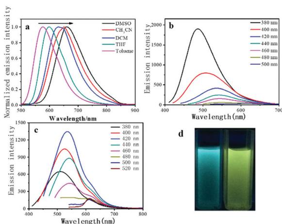
Fig. 5 (a) Normalized room temperature emission spectra of **1** with 467 nm excitation in different solvents; (b and c) emission spectra of **D-1** and **D-2** at different excitations ranging from 380 to 520 nm with a 20 nm increase in each step; (d) the photos of **D-1** and **D-2** under the irradiation of UV light at 365 nm.
