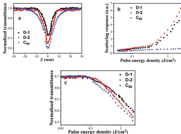
Fig. 7 (a) Open-aperture Z-scan curves, (b) scattering response, (c) optical limiting performance of **D-1**, **D-2** and **C<sub>60</sub>** with the same linear transmittance of 70% to 4 ns, 532 nm optical pulses.
