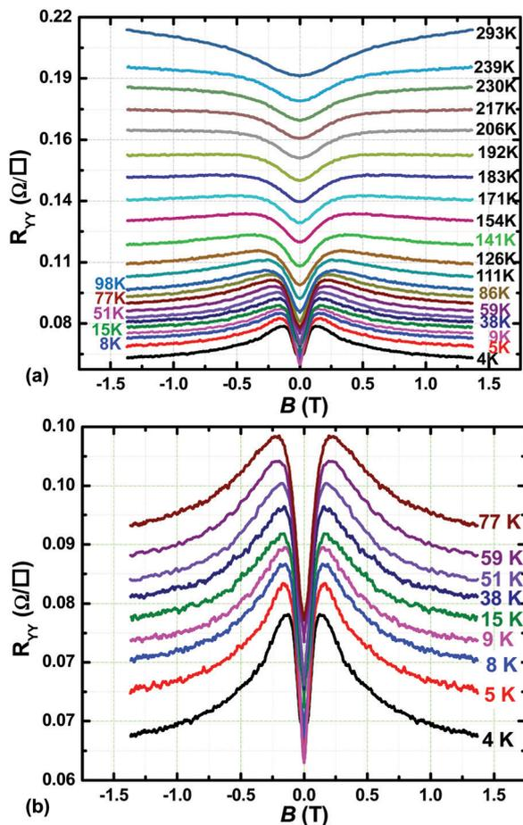
Fig. 13 (a)  $R_{YY}$  vs.  $B$ , up to  $B = \pm 1.4$  T, parametrized in  $T$  for  $T = 4$  K to  $T = 293$  K. (b)  $R_{YY}$  vs.  $B$ , up to  $B = \pm 1.4$  T, parametrized in  $T$  for  $T = 4$  K to  $T = 77$  K. The data illustrate the gradual evolution of the unique magnetoresistance with  $T$ , with magnetoresistance persisting to room temperature.
