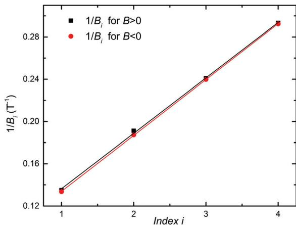
Fig. 11 Positions in inverse  $B$  of the maxima in the Shubnikov-de Haas oscillations ( $B_i$ ) for  $B > 0$  and  $B < 0$ , vs. maxima indices (with an arbitrary offset). The slopes, identical within a small error bar, yield the areal density of the carriers responsible for the oscillations, confirming the existence of higher-mobility carriers with areal density  $9.20 \times 10^{15} \text{ m}^{-2}$ .
