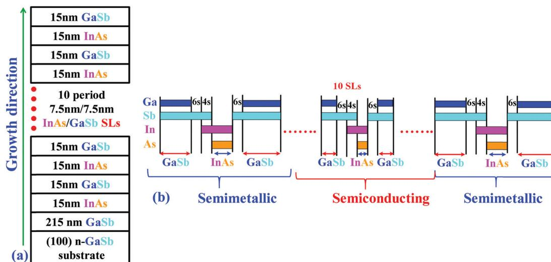
**Fig. 2** (a) Schematic diagram of the InAs/GaSb double SL structure, (b) MBE shutter sequence used during the growth of (a). A 2.13 Å InSb interfacial layer is incorporated at the InAs-on-GaSb heterointerface and  $Sb_2$  soaking is used at the InAs/GaSb heterointerface, respectively. An equal number of InAs and GaSb layers were selected such that the entire layer structure is strain-balanced. The same shutter sequences were used in both semimetallic and semiconducting heterointerfaces.
