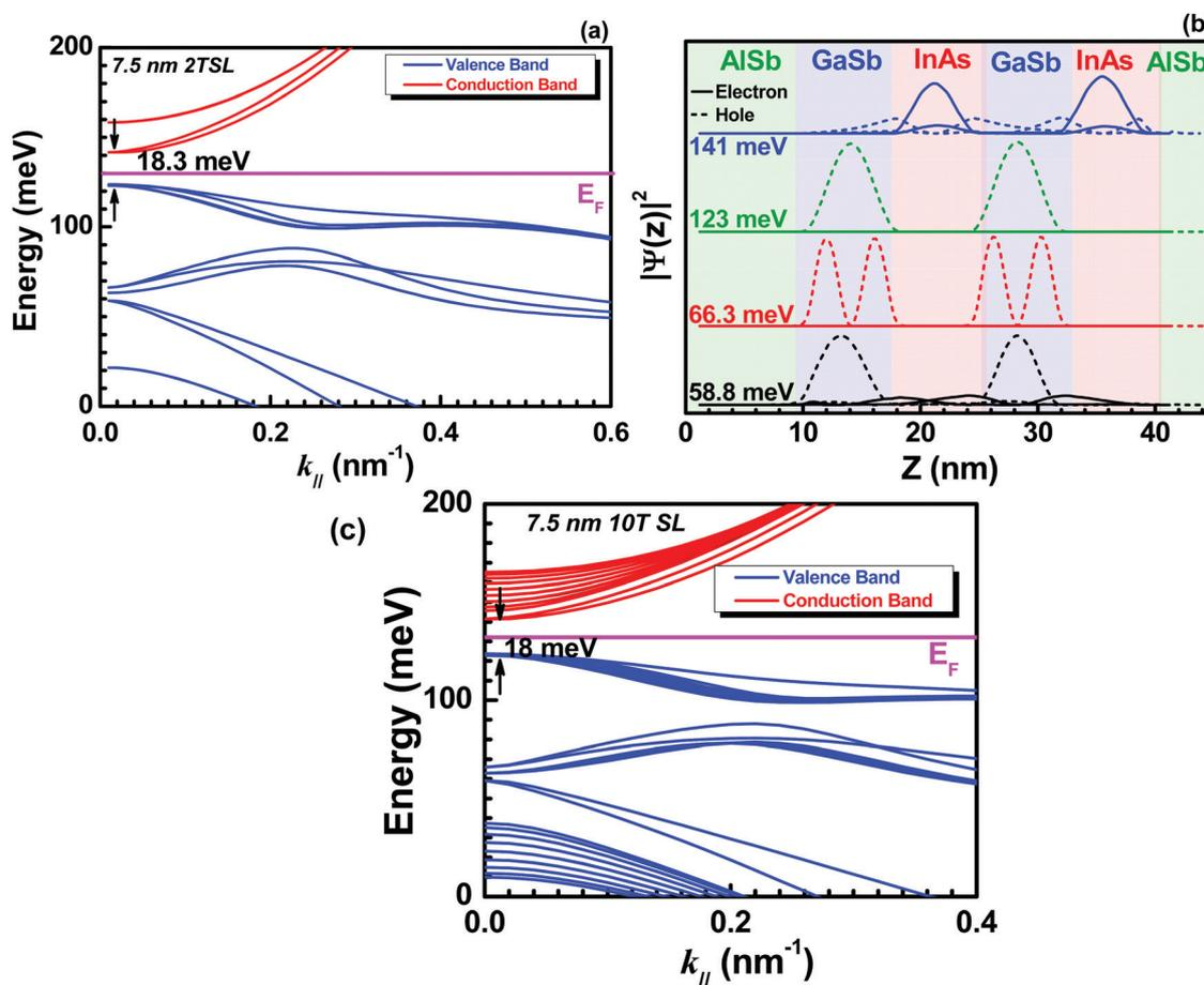
**Fig. 7** (a) Calculated electronic band structure for a 7.5 nm InAs/7.5 nm GaSb two-period superlattice inserted between two 20 nm AlSb barrier layers, (b) normalized probability density  $|\psi(z)|^2$  for the zone center states of the same structure, and (c) 7.5 nm 10 period superlattice structure, respectively. A positive energy gap of  $\sim 18$  meV was extracted, indicating the formation of a normal gap under this superlattice periodicity.
