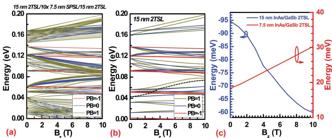
Fig. 9 Calculated band structure showing Landau levels for (a) experimentally realistic 15 nm 2T SL/10 × 7.5 nm SPSSL/15 nm 2T SL and (b) 15 nm 2T SL structure with magnetic field  $B_z$ , respectively. (c) Energy gap as a function of magnetic field for the 7.5 nm InAs/7.5 nm GaSb (red) and 15 nm InAs/15 nm GaSb (blue) 2T SL structures.
