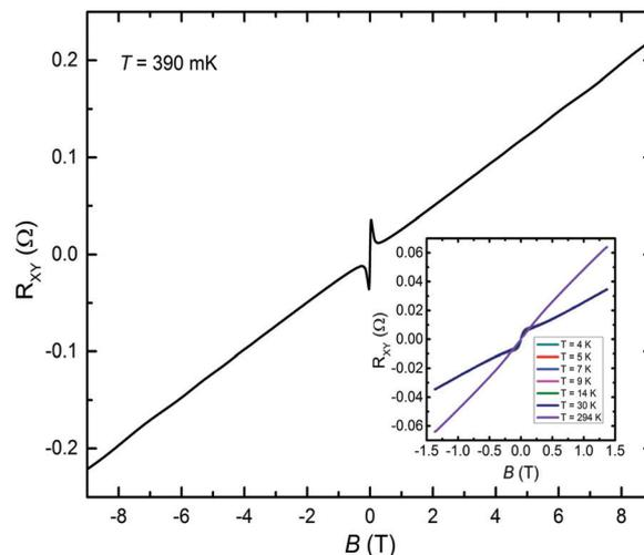
Fig. 12 Hall resistance (component  $R_{XY}$  of the magnetoresistance matrix) up to  $B = \pm 9$  T, obtained at  $T = 390$  mK. The inset shows  $R_{XY}$  parametrized in  $T$  for  $4 \text{ K} \leq T \leq 294 \text{ K}$  over  $B = \pm 1.4$  T. Deviations from linearity of  $R_{XY}$  vs.  $B$  are ascribed to intermixing with  $R_{XX}$  and  $R_{YY}$ .
