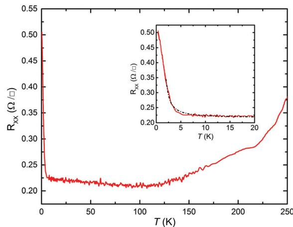
Fig. 14 Temperature dependence of  $R_{XX}$  for  $380 \text{ mK} < T < 250$  K. The inset shows the dependence on  $T$  for  $380 \text{ mK} < T < 20$  K to emphasize the pronounced rise in  $R_{XX}$  for  $T < 5$  K. In the inset the solid line represents data, and the dashed line a fit to activation across an energy gap.
