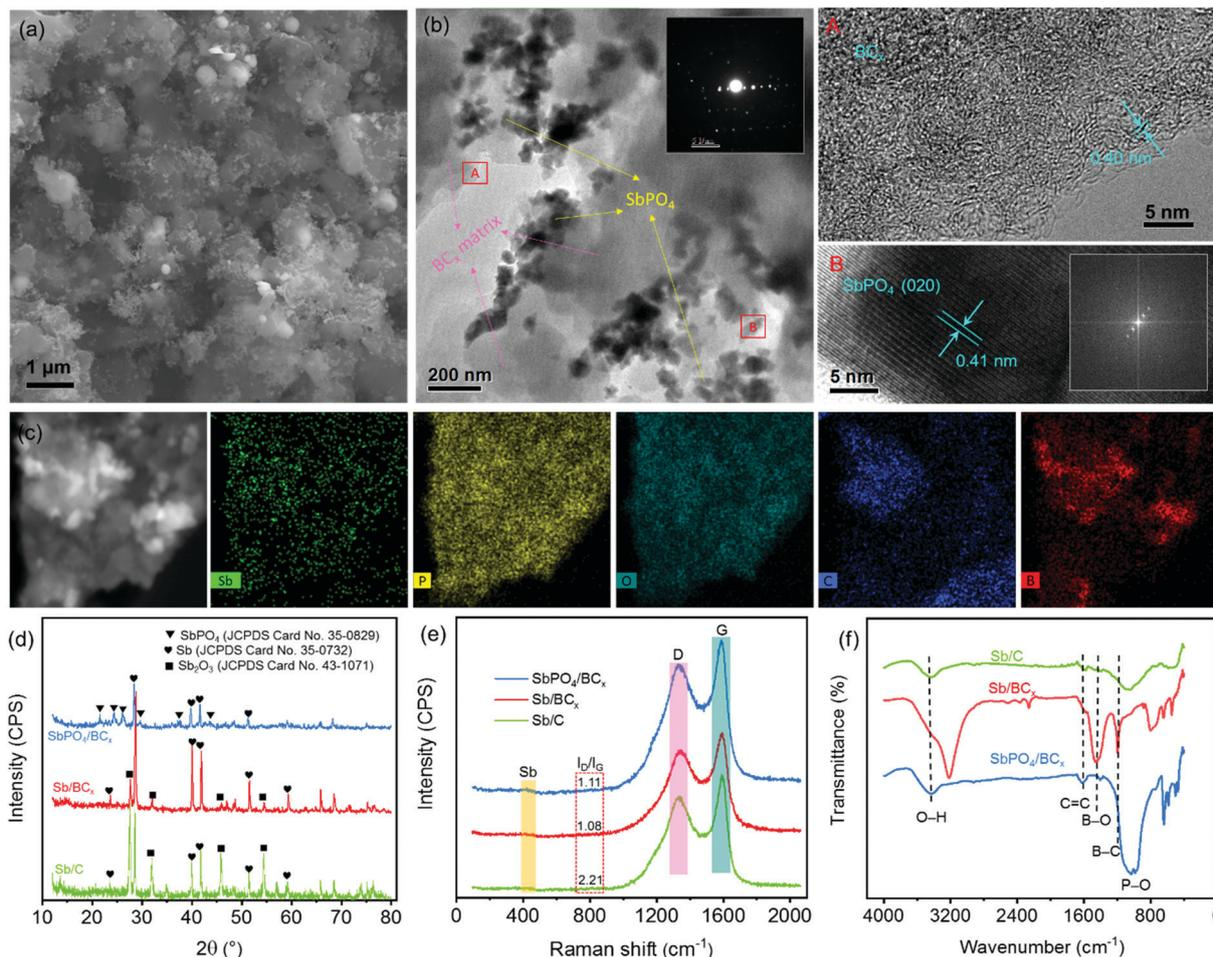
Fig. 3 SEM image (a), TEM and HRTEM images (b), and scanning TEM image with the corresponding EDS mappings of the Sb, P, O, C and B elements (c) of the  $\text{SbPO}_4/\text{BC}_x$  composite; (d) XRD patterns, (e) Raman spectra and (f) FT-IR spectra of the  $\text{SbPO}_4/\text{BC}_x$ ,  $\text{Sb}/\text{BC}_x$  and  $\text{Sb}/\text{C}$  samples. The two insets present the SAED pattern and the FFT pattern of the HRTEM image.
