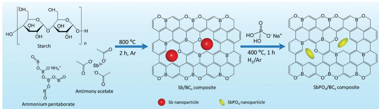
Fig. 1 Schematic illustration of the preparation process for the SbPO<sub>4</sub>/BC<sub>x</sub> composite.
