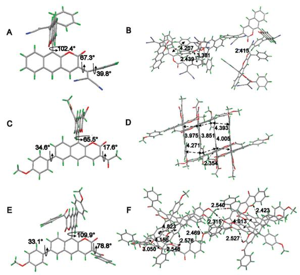
Fig. 2 Single-crystal structures of (A) **2b**, (C) **1c** and (E) **2c** and the molecular packing of (B) **2b**, (D) **1c** and (F) **2c**. Carbon, hydrogen, nitrogen and oxygen atoms are shown in grey, green, blue, and red, respectively. The single-crystal data can be found in the CCDC, the deposition numbers of **2b**, **1c** and **2c** are 1907970, 1907963 and 1907968, respectively.
