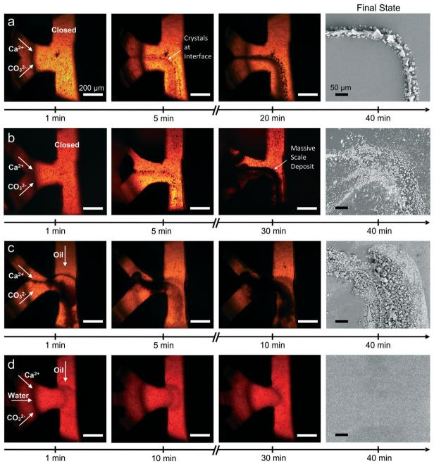
Fig. 3 Time-resolved images of the T-junction during continuous flow experiments at (a) ambient and (b) elevated temperatures and segmented flow experiments (c) without a buffer flow and (d) with a buffer flow and a nucleating agent. The last panels display SEM micrographs of the final state of the T-junction after the respective experiment. Scale bars are 200 μm in optical images and are 50 μm in SEM images.
