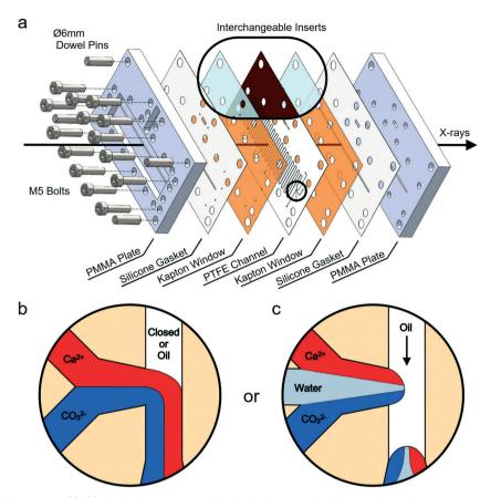
Fig. 1 (a) 3D computer-aided design (CAD) of the insert-based XRD device in an exploded view displaying the laser-cut inserts and other device components. The inset demonstrates the ability to exchange window and channel inserts. (b) The 1st design of the T-junction utilised for continuous flow or segmented flow. (c) The 2nd design of the T-junction used for providing a buffer (water) flow between reagents in segmented flow experiments.
