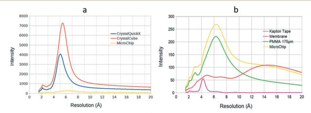
Fig. 7 a) Background scattering intensity as a function of resolution (Å) for the microfluidic chip developed in the present work and conventional crystallization plates (CrystalQuickX and CrystalCube). b) Background scattering intensity as a function of resolution (Å) from the materials composing the microfluidic assembly (2 × 175 μm thick PMMA sheet, ~20 μm thick Kapton tape and ~40 μm thick RC dialysis membrane).
