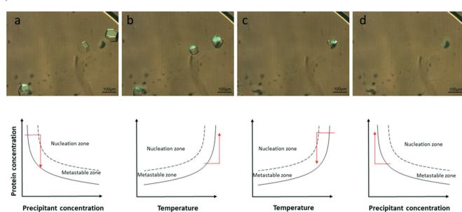
Fig. 4 Crystallization and dissolution experiment performed on-chip via the micro-dialysis method using  $\sim 30$  mg mL<sup>-1</sup> lysozyme. a) Nucleation and growth at 293 K, NaCl 0.75 M. b) Dissolution at 300 K, NaCl 0.75 M. c) Fast nucleation at 293 K, NaCl 0.75 M. d) Dissolution at 293 K, NaCl 0.75 M
