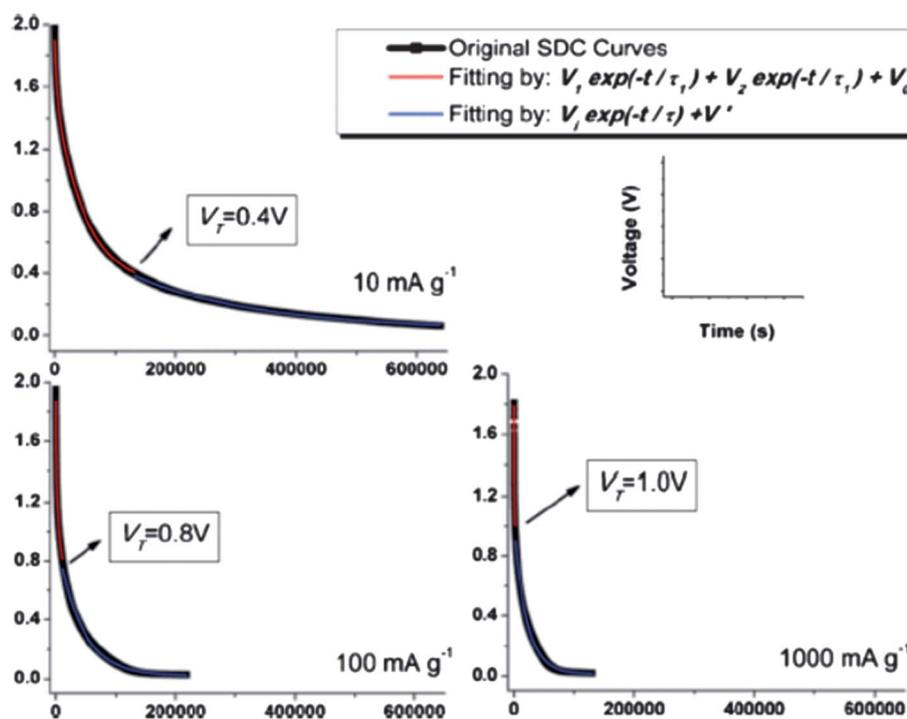
Fig. 11 Experimental SDC curves (black) and the fitting curves in DPD model (red) and SPD model (blue) marked with transition voltage  $V_T$ . Reproduced with permission from ref. 90 ©2011, The Royal Society of Chemistry.
