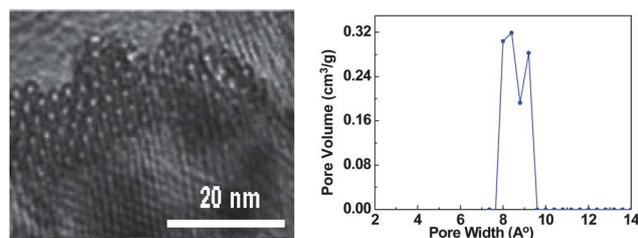
**Fig. 2** Distribution of the nanotube diameter from SEM image (left) and BET measurement (right).
