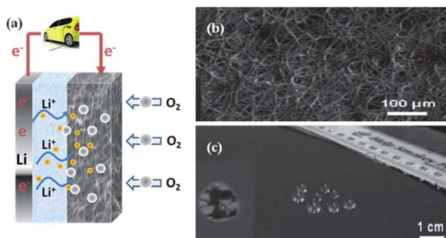
**Fig. 17** (a) The scheme of Li-O<sub>2</sub> batteries. (b) The SEM image showing micro-to-meso-porous structure of SWNT macro-films. (c) The photograph of the hydrophobic surface of the SWNT macro-films. (b) and (c) are reproduced with permission from ref. 37 ©2007, The Royal Society of Chemistry.
