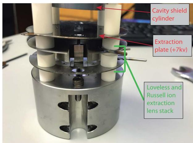
**Fig. 4** An image of the Loveless and Russell ion extraction source used in this work. In order of top to bottom, the tip of the grounded cavity shield cylinder is exposed at the top of the image (with no cavity installed), followed by the +7 kV extraction plate, then the  $x$ -symmetry plates of the Loveless and Russell source, followed by the  $z$ -symmetry plates. The bottom block contains the two collimator slits and is the original part of the 15-inch mass spectrometer.
