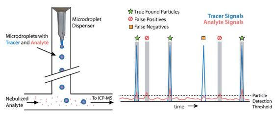
Fig. 3 Schematic diagram of a generic tracer-analyte experiment with microdroplets. Low-abundance "analyte" species in the microdroplets are treated as analyte particles and measured via sp-ICP-TOFMS. The accuracy of analyte particle detection is assessed based on the presence or absence of tracer signal concurrent with the found analyte particle signals.
