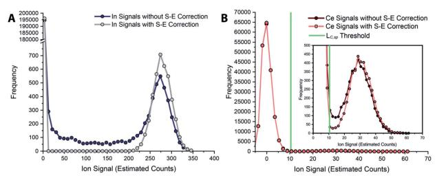
Fig. 6 Histograms of tracer (A) and analyte (B) signals without and with split-event correction. Signals from both datasets are background subtracted.
