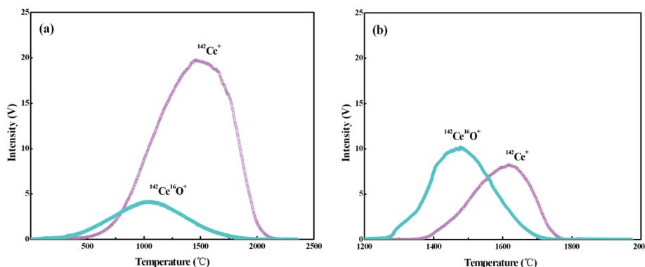
Fig. 2 Intensities of  $^{142}\text{Ce}^+$  and  $^{142}\text{Ce}^{16}\text{O}^+$  as a function of the temperature: (a) FPIE filament; (b) traditional double Re filaments. Approximately  $1\ \mu\text{g}$  Ce was loaded on the filament, and the Faraday cup configuration is shown in Line 3 of Table 3.
