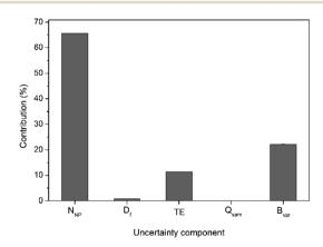
Fig. 3 Typical uncertainty budget for dynamic mass flow method, using 30 nm Au NP as an example.  $N_{\rm NP}$  is the number of particles detected in time scan,  $D_{\rm f}$  is sample dilution factor, TE is the transport efficiency,  $Q_{\rm sam}$  is the sample mass flow and  $B_{\rm var}$  is the batch-to-batch variability.
