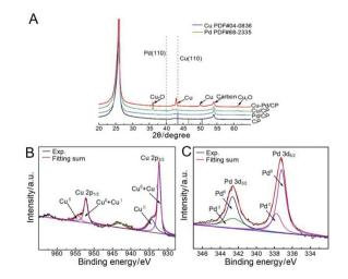
Fig. 2 (A) XRD patterns of Cu-Pd/CP, Cu/CP, Pd/CP, and CP; XPS spectra of (B) Cu 2p and (C) Pd 3d levels of catalysts.
