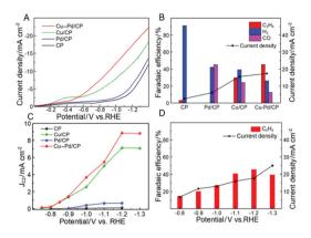
Fig. 3 (A) LSV curves of various electrodes with a scan rate of 50 mV $^{-1}$ ; (B) the FE of  $C_2H_4$  at -1.2 V (vs. RHE) over various electrodes; (C) partial current density of  $C_2H_4$  over various electrodes at different applied potentials; (D) the FE and current density of  $C_2H_4$  over Cu-Pd/CP at different applied potentials in  $CO_2$ -saturated 0.1 M KCl solution.
