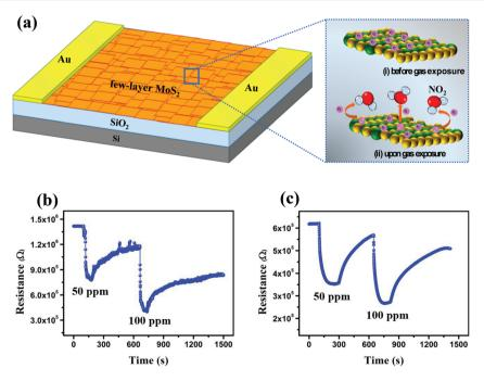
Fig. 7 (a) Schematic illustration of the sensing behavior of the fabricated device based on the charge-transfer mechanism, and the sensing performance of the MC6 sample against 50 and 100 ppm NO2 at 50 °C (b) and 100 °C (c).
