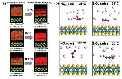
Fig. 9 (a) Field density distribution of a 5% NO<sub>2</sub> and 95% Ar mixture on the predominant (002) surface of molybdenite-2H. Atoms: sulphur, yellow; and molybdenum, light blue. Isosurface:  $NO_2$ , green; and Ar, red. (b) Close contacts (less than 3.7 Å) of  $NO_2/NO_2$  species on the predominant (002) surface of molybdenite-2H. Atoms: sulphur, yellow; molybdenum, light blue; nitrogen, dark blue; oxygen, red; and argon, grey.
