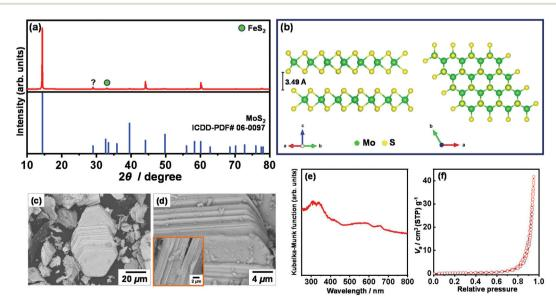
Fig. 2 (a) XRD pattern, (b) side and top views of the crystal structure of molybdenite (2H polytype), (c and d) BSE-SEM images, (e) UV-vis DRS spectrum, and (f) N<sub>2</sub> adsorption-desorption isotherm of molybdenite concentrate.
