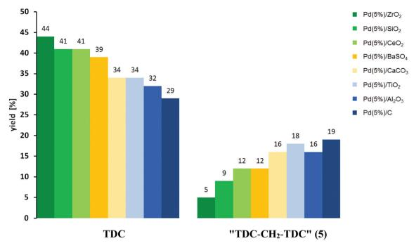
Fig. 6 Influence of the support material on the palladium-catalysed oxidative carbonylation of TDA with MF. Reaction conditions: 485 mmol MF; 0.5 mmol NaOMe; 0.011 mmol Pd; 0.6 mmol NaI; 5 mmol TDA in 5 mL MeOH; 140 °C; reaction time 4 h. Quantified by HPLC-analysis using external standard solutions.
