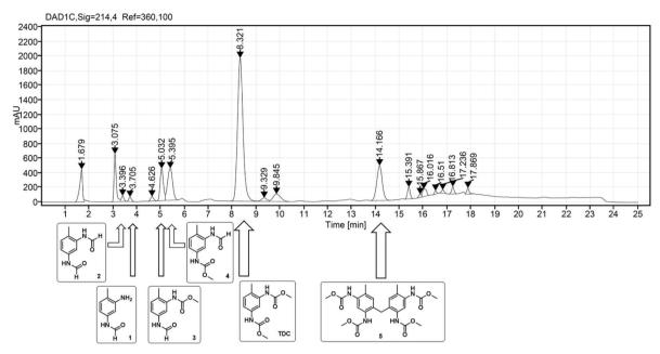
Fig. 1 HPLC analysis of a typical reaction mixture of the oxidative carbonylation of TDA with MF: assignment of TDC and the identified side products 1–5 by UV detection at 214 nm.
