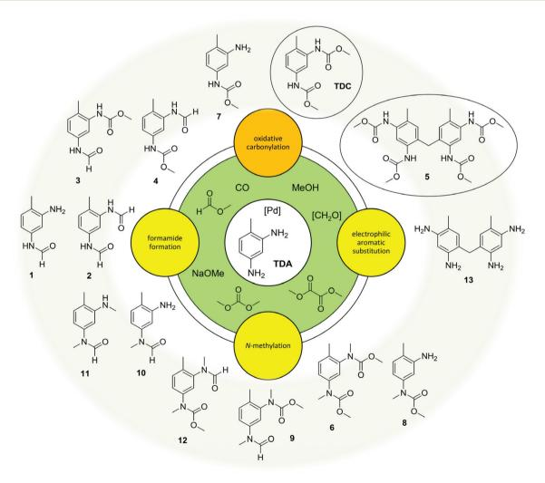
Fig. 4 Oxidative carbonylation of TDA with MF: complex reaction network.
