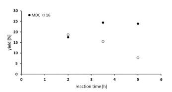
Fig. 7 Oxidative carbonylation of MDA with MF: dependence of reaction time on the yield of MDC and 16 [69–72 bar CO; 3.6–4.5 vol%  $O_2$ ; MF (485 mmol); NaOMe (0.5 mmol); Pd(5%)/Al $_2O_3$  (0.011 mmol Pd); NaI (0.6 mmol); MDA (2.5 mmol) in MeOH (5 mL)].
