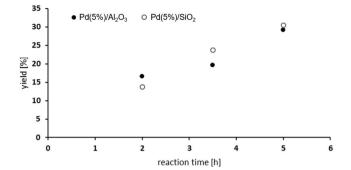
Fig. 8 Oxidative carbonylation of 17 with MF: dependence of reaction time on the yield of 18 [65-81 bar CO; 4.2-5.2 vol%  $O_2$ ; 485 mmol MF; 0.5 mmol NaOMe; 0.011 mmol Pd; 0.6 mmol NaI; 5 mmol 17 in 5 mL MeOHI.
