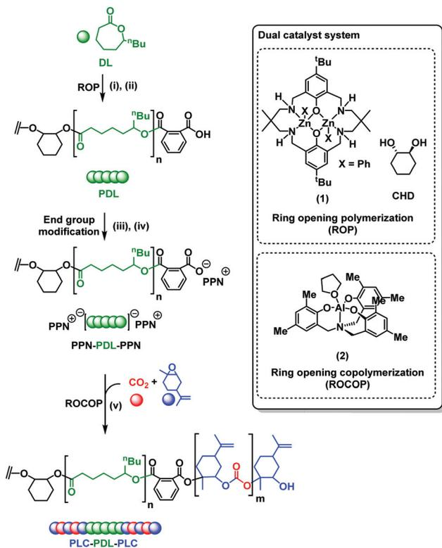
**Scheme 1** Block polymer synthesis. (i) 1,2-cyclohexane diol (CHD), ε-decalactone (DL), 2 h, 100 °C, toluene. (ii) Phthalic anhydride (PA), 16 h, 100 °C, molar ratio: [1]/[CHD]/[PA]/[DL] = 1/4/100/350–1000. (iii) NaOH, 2 h, 25 °C, chloroform. (iv) PPNi, 2 h, 40 °C. Molar ratio: [diacid end group]/[NaOH]/[PPNi] = 1/1/1. (v) [2]: [PPN-PDL-PPN]: [LO] = 1 : 0.25 : 125 (LO used as monomer and solvent), 24 h, 20 bar CO<sub>2</sub>, 45 °C.
