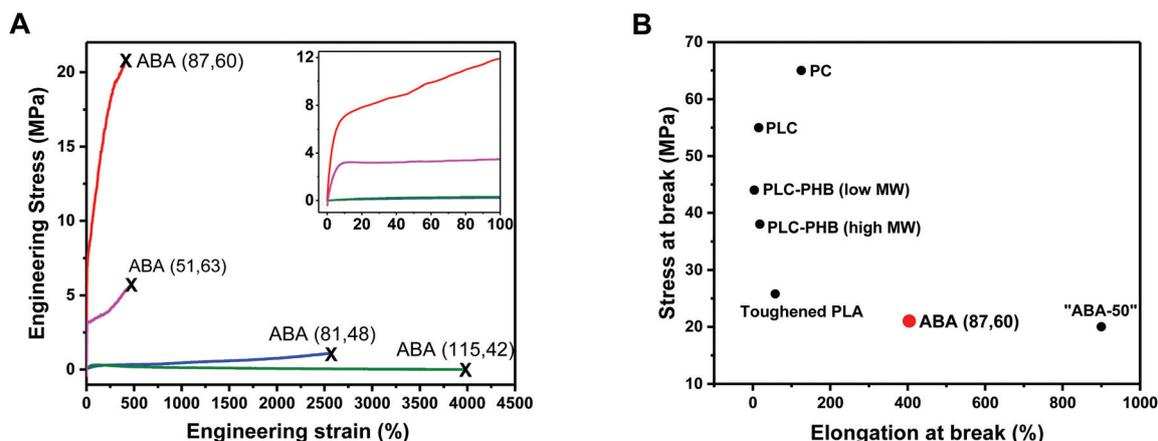
**Fig. 3** Mechanical Properties of PLC-*b*-PDL-*b*-PLC triblock polymers. (A) Stress-strain curves for uniaxial extension measurements. Failure points marked with an "X". Inset: enlargement of the 0–100% strain region. (B) Ashby plot of tensile strength vs. elongation at break allowing comparison of the properties of ABA (87,60) with commercial and literature samples (see ESI Table S1† for further details on samples used in comparison).
