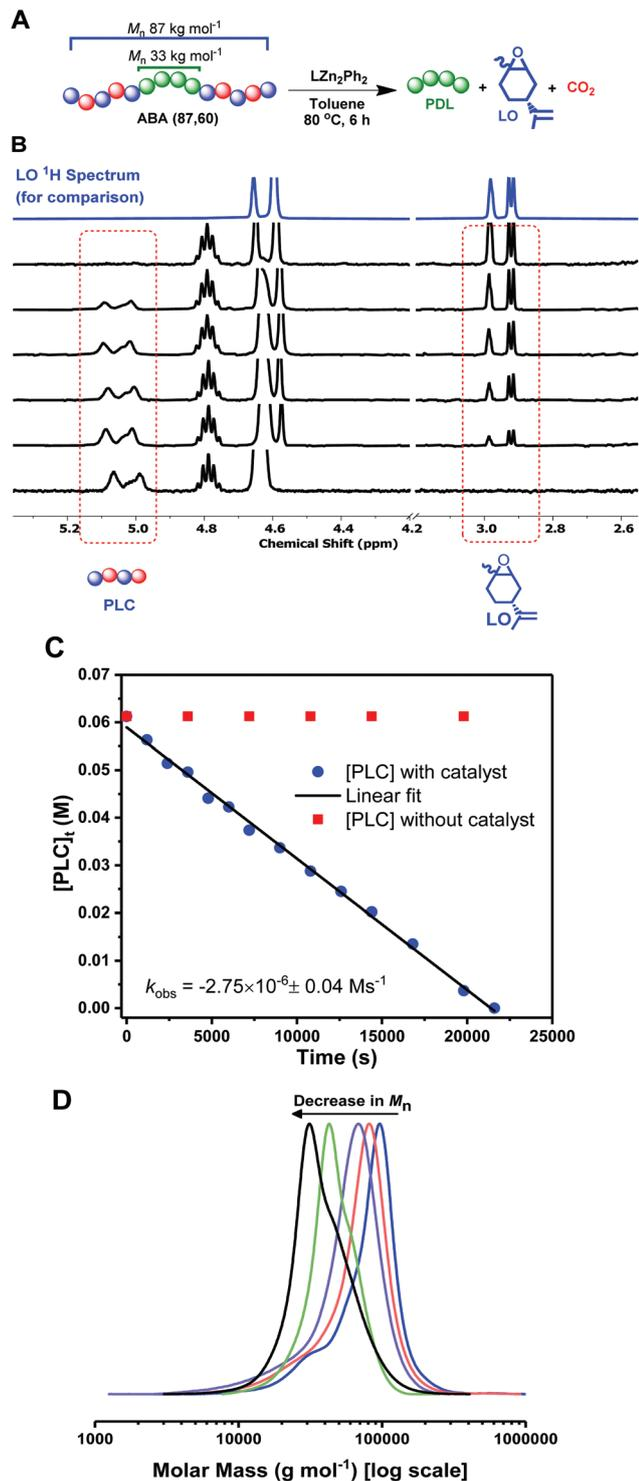
Fig. 4 Depolymerization reactions of ABA (87,60). (A): 1.6 mM of **1**; (B) Stacked  $^1\text{H}$  NMR spectra ( $\text{CDCl}_3$ ) taken at various timepoints throughout the depolymerization (LO  $^1\text{H}$  NMR spectrum is added for comparison); (C) Kinetic analysis with catalyst **1** (blue circles) and no catalyst (red squares); (D) SEC analysis (THF eluent, vs. PS standards) of aliquots taken at various time-points (see also Fig. S19 $\dagger$ ).
