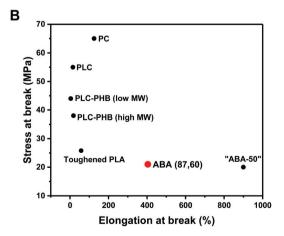
Fig. 3 Mechanical Properties of PLC-*b*-PDL-*b*-PLC triblock polymers. (A) Stress–strain curves for uniaxial extension measurements. Failure points marked with an "X". Inset: enlargement of the 0–100% strain region. (B) Ashby plot of tensile strength *vs.* elongation at break allowing comparison of the properties of ABA (87,60) with commercial and literature samples (see ESI Table S1† for further details on samples used in comparison).
