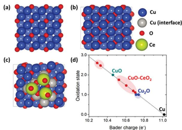
**Fig. 5** Top view of the optimized geometries of (a)  $\text{Cu}_2\text{O}$ , (b)  $\text{CuO}$ , and (c)  $\text{CuO-CeO}_2$ . (d) Oxidation states of surface Cu atoms obtained by Bader charge analysis. Only the surface Cu atoms adjacent to  $\text{CeO}_2$  (denoted as grey balls in (c)) are considered for the Bader charge analysis of  $\text{CuO-CeO}_2$ . In (d), black, blue, cyan, and red colors represent Cu,  $\text{Cu}_2\text{O}$ ,  $\text{CuO}$ , and  $\text{CuO-CeO}_2$ , respectively.
