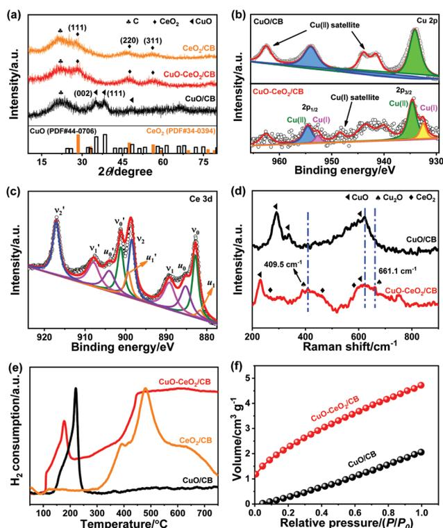
**Fig. 1** (a) XRD patterns of  $\text{CeO}_2/\text{CB}$ , CuO/CB, and CuO– $\text{CeO}_2/\text{CB}$ . (b) Cu 2p XPS spectra of CuO/CB and CuO– $\text{CeO}_2/\text{CB}$ . (c) Ce 3d XPS spectrum of CuO– $\text{CeO}_2/\text{CB}$ . (d) Raman spectra of CuO/CB and CuO– $\text{CeO}_2/\text{CB}$ . (e)  $\text{H}_2$ -TPR profiles of  $\text{CeO}_2/\text{CB}$ , CuO/CB, and CuO– $\text{CeO}_2/\text{CB}$ . (f)  $\text{CO}_2$  adsorption isotherms of CuO/CB and CuO– $\text{CeO}_2/\text{CB}$ .
