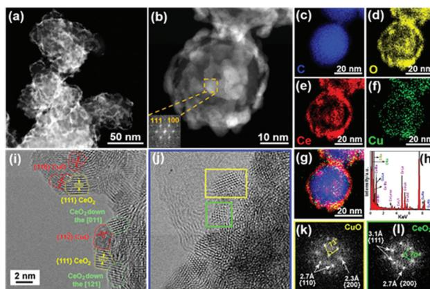
**Fig. 2** (a and b) HAADF-STEM images of CuO– $CeO_2$ /CB. The inset in image (b) shows the corresponding FFT of CuO– $CeO_2$ /CB. EDS elemental maps of (c) C, (d) O, (e) Ce, (f) Cu, and (g) overlay of C (blue), Ce (red), and Cu (green) over the region shown in image (b), along with corresponding EDS spectrum (h). (i) HRTEM image of CuO– $CeO_2$ /CB. (j–l) Magnified image of the blue rectangle in image (i) and FFTs of the regions encased by the yellow and green rectangles in image (j).
