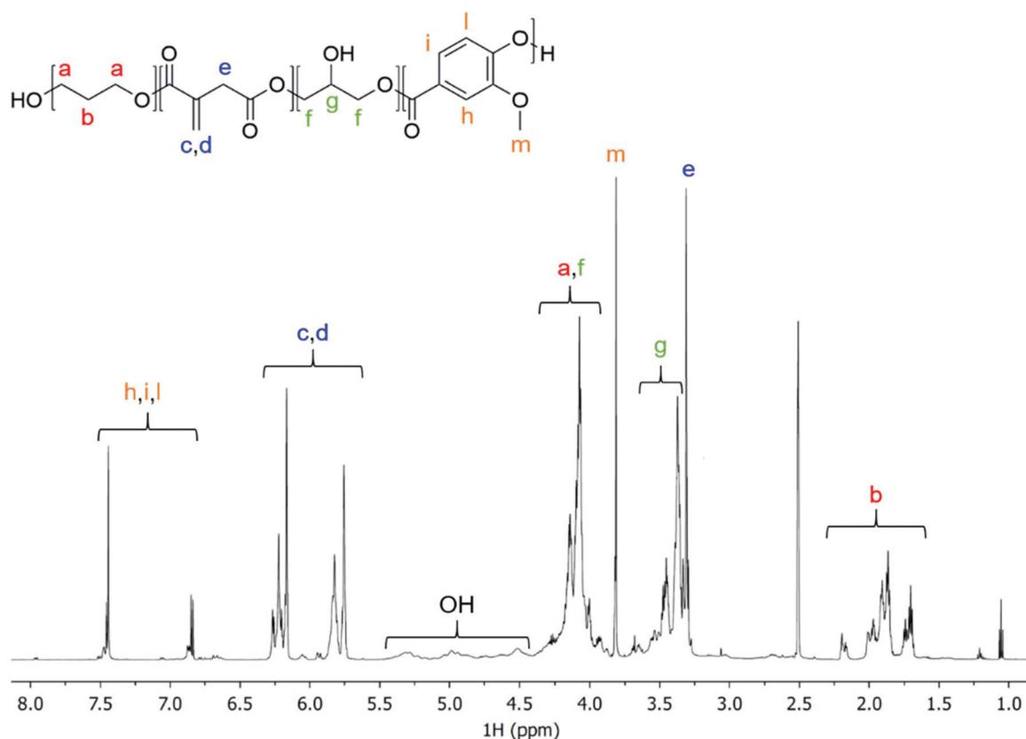
Fig. 2  $^1\text{H}$  NMR spectrum (600 MHz, DMSO- $d_6$ ) of PPGIV, with the assignment of peaks to the related monomers or functional groups.
