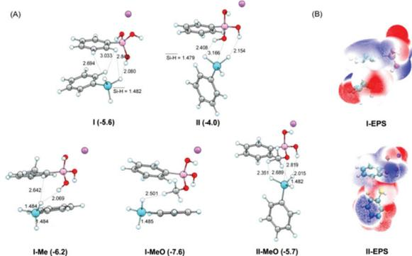
**Fig. 3** DFT-calculated interaction modes. (A) Optimized complex structures of sodium aryl borates (**3j**, **3k**, and **3o**) with phenylsilane at the M06-2X-D3/6-311G(d, p) level of theory in solvent. Values in parenthesis denote the binding energies (in kcal mol<sup>-1</sup>) calculated at the DSD-PBEP86/def2-TZVPP level in solvent. Bond lengths are in Å. (B) Electrostatic potential map for the catalyst-silane interaction.
