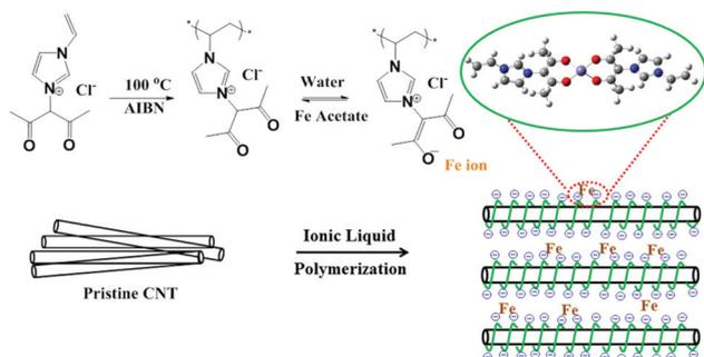
**Fig. 1** Schematic illustration of the designed catalyst. Schematic illustration of the fabrication process of the Fe-PIL/CNTs. The model structure in the green cycle shows the coordinated sphere of the isolated iron species in the final product.
