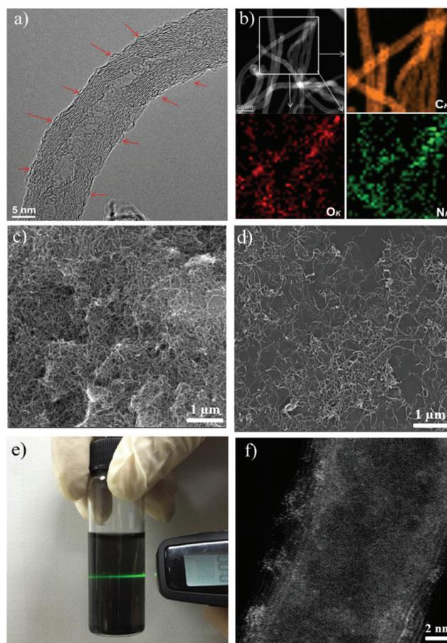
**Fig. 2** (a) HRTEM image of the PIL/CNTs (red arrows point to the PIL layer). (b) HAADF STEM-EDS mapping of C, N, and O, as labelled, measured in the white box of the PIL/CNTs. SEM images of the (c) pristine CNT and (d) PIL/CNTs. (e) Photograph images of PIL/CNT dispersions in water (the weight of the sample is 1 mg). (f) The STEM image of the sample, which shows the distribution of the iron sites on the CNT surface.
