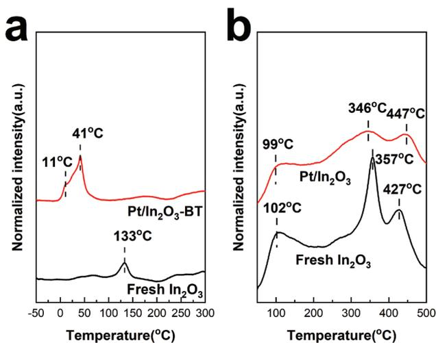
**Fig. 6** (a) H<sub>2</sub>-TPR profiles and (b) CO<sub>2</sub>-TPD profiles of the Pt/In<sub>2</sub>O<sub>3</sub> and pure In<sub>2</sub>O<sub>3</sub> catalysts.
