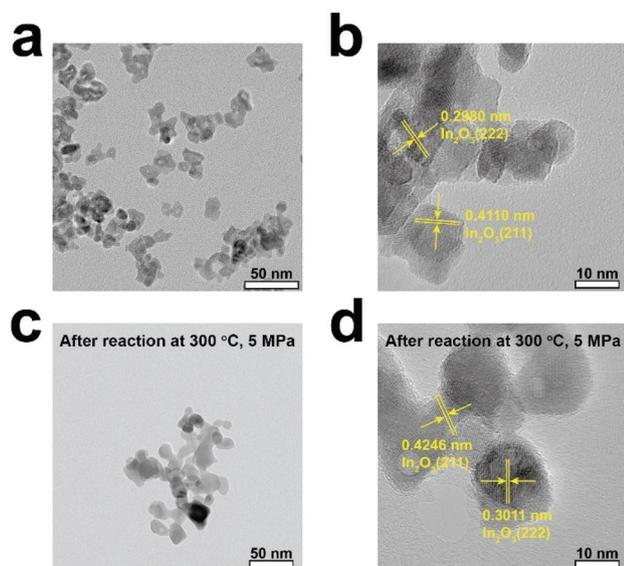
**Fig. 4** TEM images of (a and b) the fresh In<sub>2</sub>O<sub>3</sub> catalyst and (c and d) the pure In<sub>2</sub>O<sub>3</sub> catalyst after reaction.
