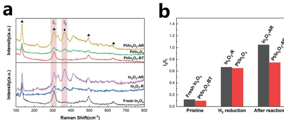
**Fig. 5** (a) Visible Raman spectra of the Pt/In<sub>2</sub>O<sub>3</sub> and pure In<sub>2</sub>O<sub>3</sub> catalysts, (b) comparison of the relative amount of the oxygen vacancies according to the I<sub>2</sub>/I<sub>1</sub> ratio. ♣ : InO<sub>6</sub> octahedron, ◆ : the stretching vibrations of In-O-In. In<sub>2</sub>O<sub>3</sub>-R represents the In<sub>2</sub>O<sub>3</sub> catalyst after hydrogen reduction (H<sub>2</sub>/N<sub>2</sub> = 1/9, molar ratio, at 200 °C for 1 h).
