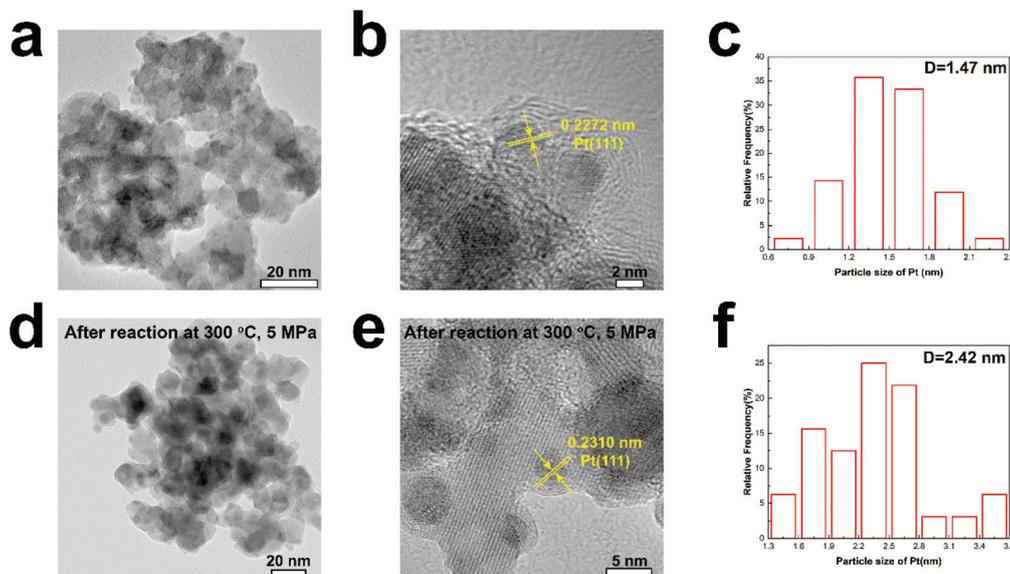
**Fig. 3** (a) and (b) TEM images of the Pt/In<sub>2</sub>O<sub>3</sub> catalyst, (c) particle size distribution for the Pt/In<sub>2</sub>O<sub>3</sub> catalyst, (d) and (e) TEM images of Pt/In<sub>2</sub>O<sub>3</sub> after reaction, and (f) particle size distribution for Pt/In<sub>2</sub>O<sub>3</sub> after reaction.
