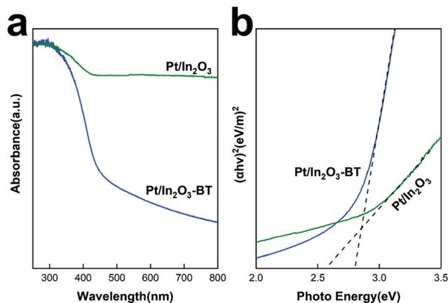
Fig. 7 (a) UV-vis absorption spectra and (b) Tauc plot of the Pt/In<sub>2</sub>O<sub>3</sub> catalyst.
