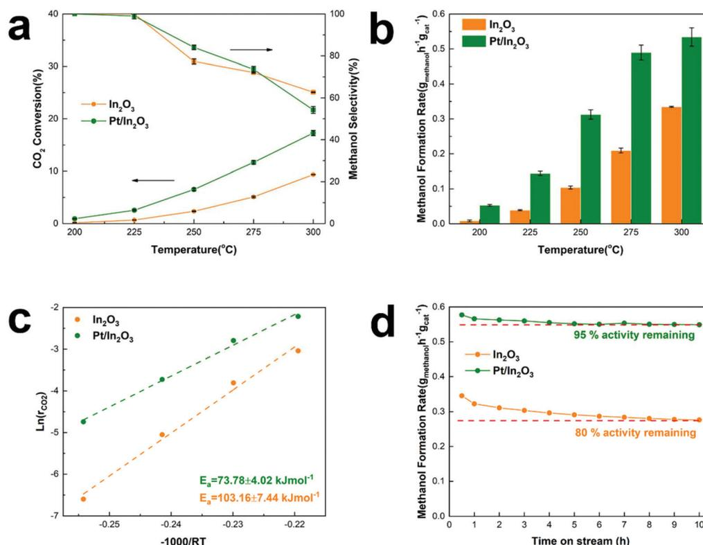
**Fig. 1** Catalytic activity tests of the Pt/In<sub>2</sub>O<sub>3</sub> and pure In<sub>2</sub>O<sub>3</sub> catalysts. (a) CO<sub>2</sub> conversion and methanol selectivity, (b) methanol formation rate as a function of reaction temperature, (c) apparent activation energy of CO<sub>2</sub> conversion and (d) methanol formation rate versus time of the catalyst in the reaction stream (TOS).
