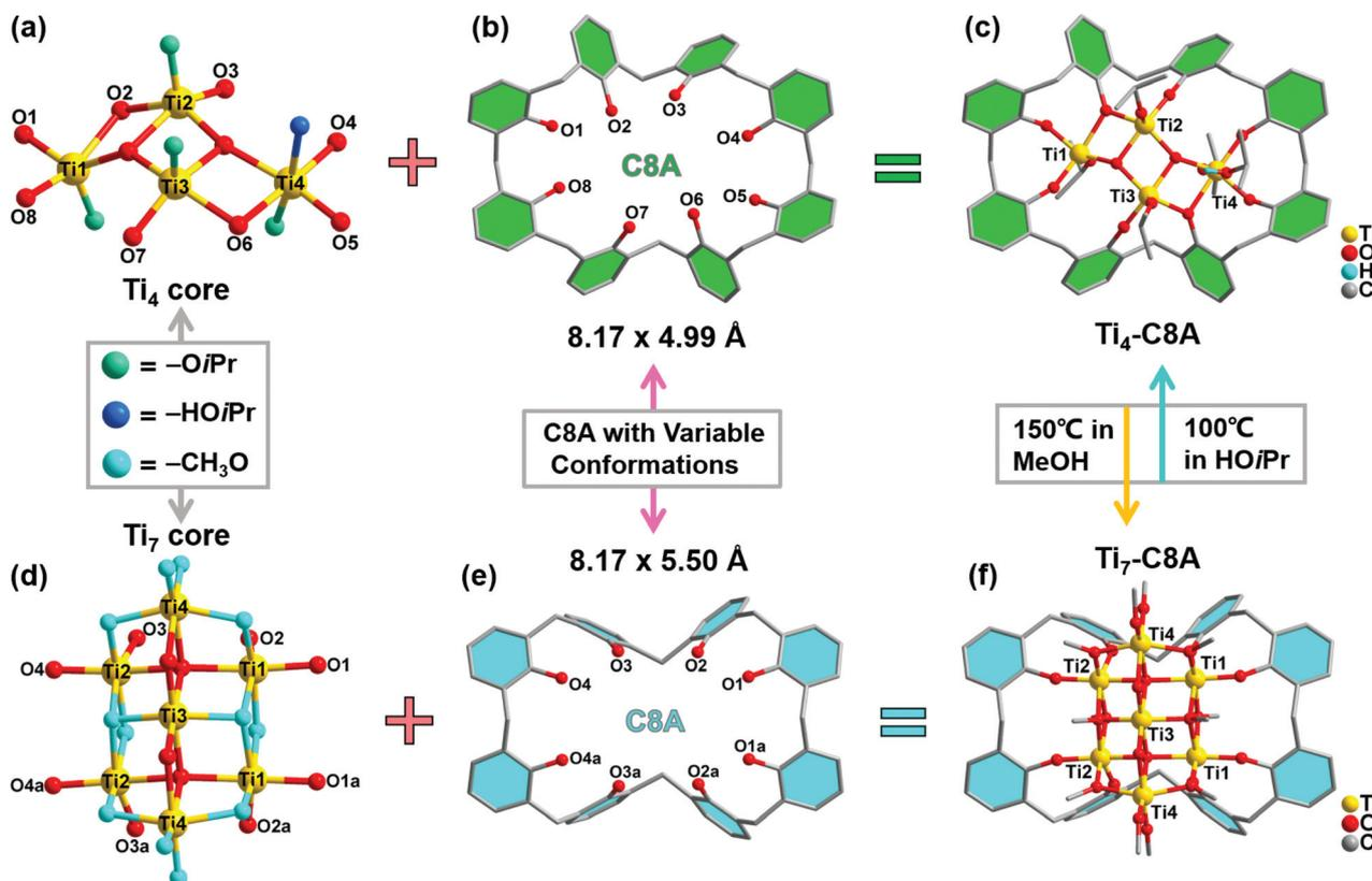
**Fig. 1** Schematic of the crystal structures of **Ti<sub>4</sub>-C8A** and **Ti<sub>7</sub>-C8A**. (a) The metal-oxo core, (b) C8A ligand (cavity of *ca.*  $8.17 \times 4.99$  Å), and (c) overall cluster structure of **Ti<sub>4</sub>-C8A**. (d) The metal-oxo core, (e) C8A ligand (cavity of *ca.*  $8.17 \times 5.50$  Å), and (f) overall cluster structure of **Ti<sub>7</sub>-C8A**. Except for the protonated  $-\text{OiPr}$  group (blue ball), all the hydrogen atoms are omitted for clarity.
