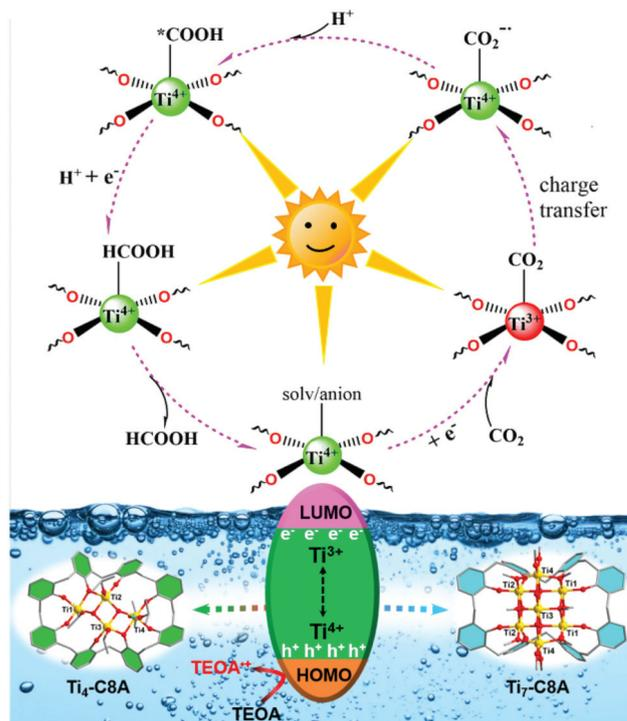
Fig. 4 The proposed photocatalytic reaction mechanism for Ti<sub>4</sub>-C8A and Ti<sub>7</sub>-C8A.
