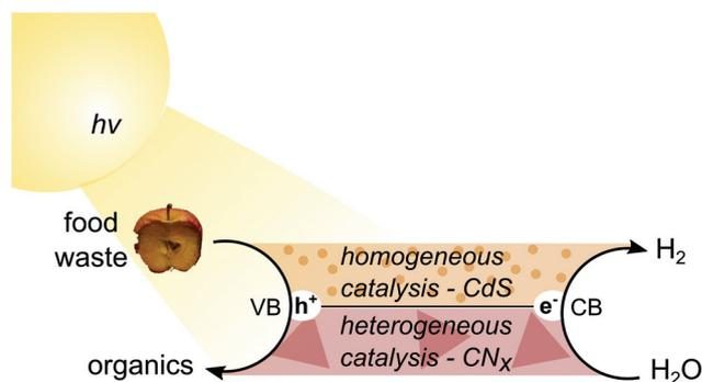
Fig. 1 Schematic diagram of food waste photoreforming over CdS/CdO<sub>x</sub> quantum dots or <sup>H2N</sup>CN<sub>x</sub>|Ni<sub>2</sub>P.
