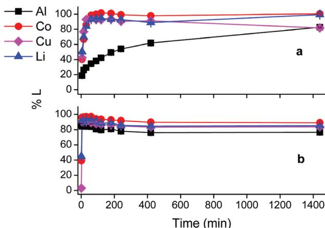
**Fig. 6** Comparison between leaching with leaching of  $\text{LiCoO}_2$  by DES and HCl solution. Top: DES leaching ( $\text{ChCl}:\text{CA } 2:1 + 35 \text{ wt\% H}_2\text{O}$ ). Bottom: Leaching with HCl  $1 \text{ mol L}^{-1}$ . Leaching parameters: S:L = 20 g  $\text{L}^{-1}$ ,  $40 \text{ }^\circ\text{C}$ , Al:  $\text{LiCoO}_2 = 12 \text{ wt\%}$ , Cu:  $\text{LiCoO}_2 = 24 \text{ wt\%}$  at a stirring rate of 900 rpm.
