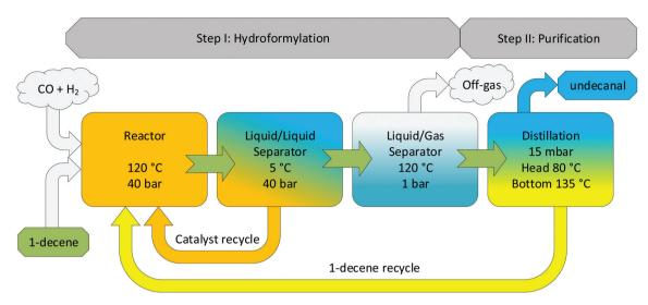
Fig. 9 Process concept for an intensified process for CD-based hydroformylation.
