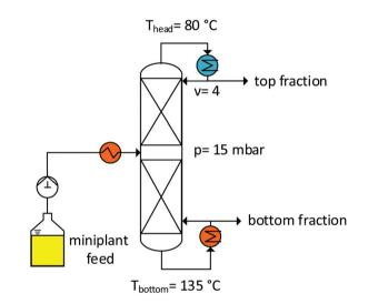
Fig. 11 Distillation column for substrate recycling.
