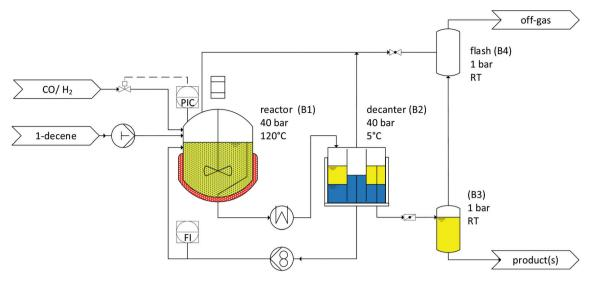
Fig. 10 Flowchart of the continuously operated miniplant.
