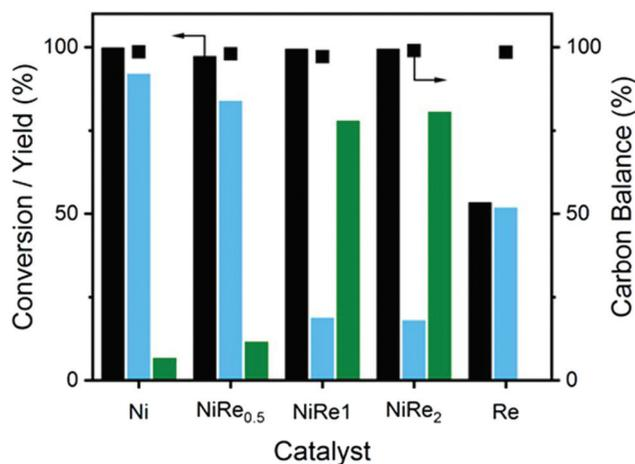
Fig. 1 Evaluation of titania-supported Ni, NiRe<sub>x</sub> and Re catalysts in the hydrogenation of aqueous 1 wt% 5-HMF solutions.
