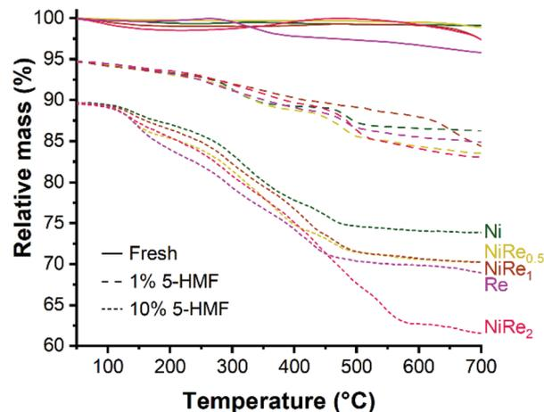
Fig. 4 TG curves showing relative mass loss of fresh and spent Ni, NiRe<sub>x</sub> and Re used for the hydrogenation of 1 wt% and 10 wt% 5-HMF. TG curve sets are offset by –5% (1 wt% 5-HMF) and –10% (10 wt% 5-HMF) for clarity.
