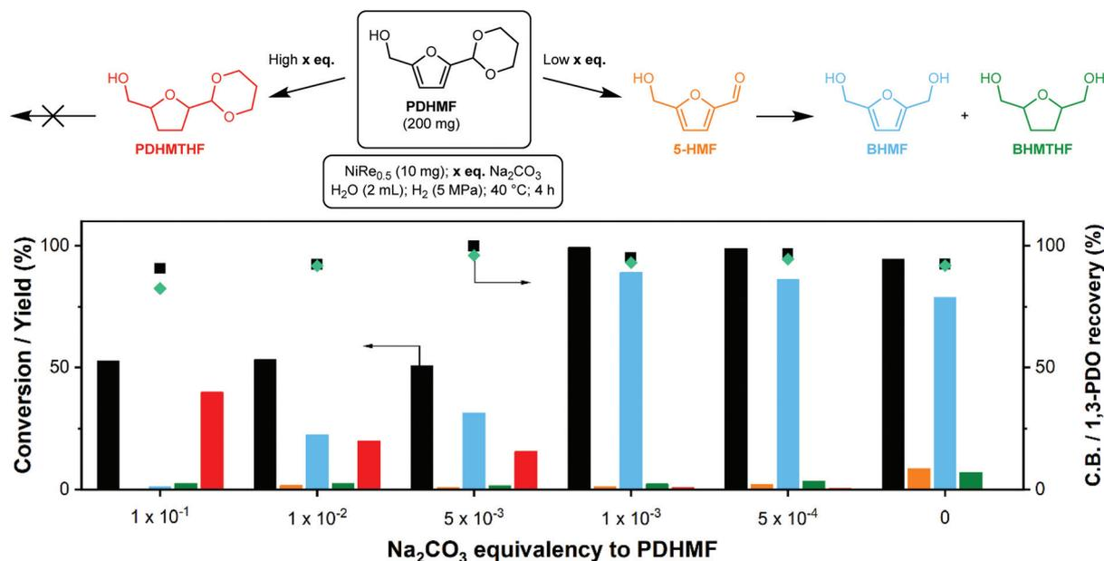
Fig. 5 Conversion and product distribution as function of Na<sub>2</sub>CO<sub>3</sub> equivalencies for the hydrogenation of aqueous 10 wt% PDHMF solutions using NiRe<sub>0.5</sub> as catalyst. Carbon balances are marked with black squares. Teal diamond markers indicate 1,3-PDO recovery as a sum of unreacted PDHMF, PDHMTf and free 1,3-propanediol. 1,3-PDO originates from deprotection of PDHMF during the course of the reaction. It is excluded from the carbon balance.
