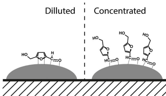
Fig. 3 Proposed 5-HMF orientations in dilute (1 wt%) and concentrated (10 wt%) solutions over NiRe<sub>1</sub> and NiRe<sub>2</sub> bimetallic catalysts.
