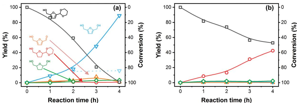
Fig. 6 Time courses of BHMF formation from PDHMF with  $\text{NiRe}_{0.5}$  using (a)  $1 \times 10^{-3}$ , and (b)  $5 \times 10^{-2}$  eq.  $\text{Na}_2\text{CO}_3$ . Lines provide guidance for the reader's eye. Reagents and conditions: Catalyst (10 mg), PDHMF (200 mg, molar ratio PDHMF/Ni = 214),  $\text{H}_2\text{O}$  (2 mL), 1-butanol (1  $\mu\text{L}$ ),  $\text{H}_2$  (5 MPa), 40  $^\circ\text{C}$ , 750 rpm. Dashed line and transparent symbols (a) show BHMF yield after catalyst removal.
