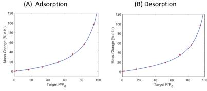
Fig. 3 Dynamic vapor sorption analysis of superabsorbent polymer Luquafleece fabric at 40 °C. (A) Adsorption isotherm followed by (B) desorption isotherm. Data are shown with a fit using the GAB model and fitting parameters are reported in Table 4.
