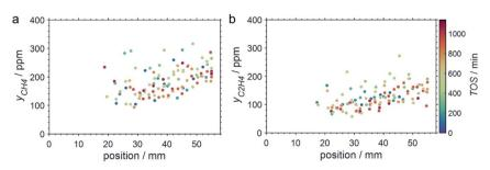
Fig. 7 Concentration profiles of (a) methane and (b) ethylene as a function of the catalyst bed length at various points in time during PDH over GaPt/SiO $_2$  SCALMS with an atomic ratio of Ga/Pt of 55 at 550 °C. Conditions of the experiment: 22 mL $_N$  min $^{-1}$  He; 3 mL $_N$  min $^{-1}$  C $_3$ H $_8$ ; WHSV 4500 mL $_N$  g $^{-1}$  h $^{-1}$ .
