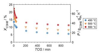
Fig. 4 Conversion of propane and productivity at the end of the catalyst bed during PDH over GaPt/SiO $_2$  SCALMS with an atomic ratio of Ga/Pt of 55 at 450–550 °C. The error bars represent the standard deviation of 6 consecutive measurements in-between profile acquisitions. Conditions of the experiment: 22 mL $_N$  min $^{-1}$  He; 3 mL $_N$  min $^{-1}$  C $_3$ H $_8$ ; WHSV 4500 mL $_N$  g $^{-1}$  h $^{-1}$ .
