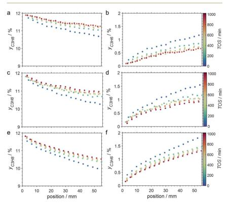
Fig. 5 Concentration profiles of propane (a, c, and e) and propylene (b, d and f) as a function of the catalyst bed length at various points in time during PDH over GaPt/SiO<sub>2</sub> SCALMS with an atomic ratio of Ga/Pt of 55 at (a and b) 450 °C, (c and d) 500 °C, and (e and f) 550 °C. Conditions of the experiment: 22 mL<sub>N</sub> min<sup>-1</sup> He; 3 mL<sub>N</sub> min<sup>-1</sup>  $C_3H_8$ ; WHSV 4500  $mL_N g^{-1} h^{-1}$ .
