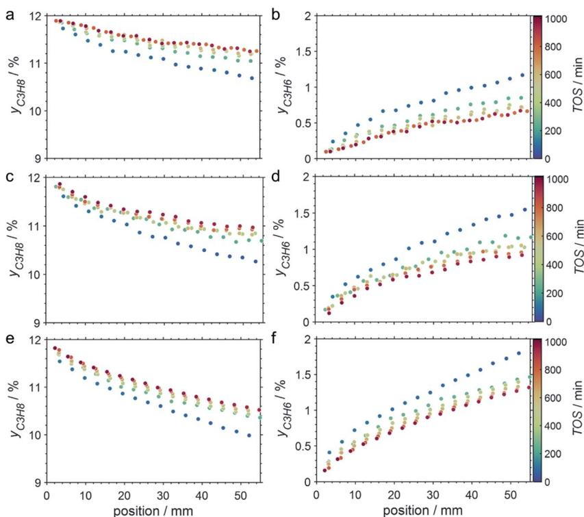
Fig. 5 Concentration profiles of propane (a, c, and e) and propylene (b, d and f) as a function of the catalyst bed length in time during PDH over GaPt/SiO<sub>2</sub> SCALMS with an atomic ratio of Ga/Pt of 55 at (a and b) 450 °C, (c and d) 500 °C, and (e and f) 550 °C. Conditions of the experiment: 22 mL<sub>N</sub> min<sup>-1</sup> He; 3 mL<sub>N</sub> min<sup>-1</sup> C<sub>3</sub>H<sub>8</sub>; WHSV 4500 mL<sub>N</sub> g<sup>-1</sup> h<sup>-1</sup>.
