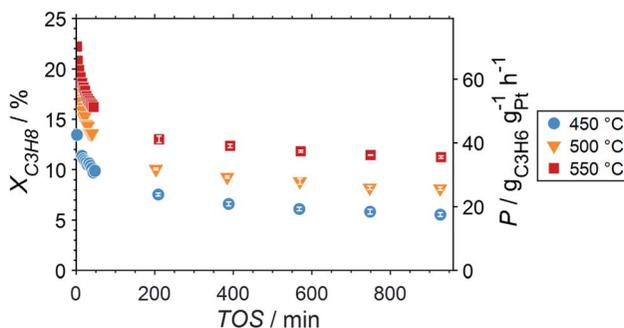
Fig. 4 Conversion of propane and productivity at the end of the catalyst bed during PDH over GaPt/SiO<sub>2</sub> SCALMS with an atomic ratio of Ga/Pt of 55 at 450–550 °C. The error bars represent the standard deviation of 6 consecutive measurements in-between profile acquisitions. Conditions of the experiment: 22 mL<sub>N</sub> min<sup>-1</sup> He; 3 mL<sub>N</sub> min<sup>-1</sup> C<sub>3</sub>H<sub>8</sub>; WHSV 4500 mL<sub>N</sub> g<sup>-1</sup> h<sup>-1</sup>.
