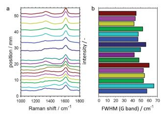
Fig. 10 (a) Spatially resolved Raman spectra of the catalyst bed after propane dehydrogenation over GaPt/Al<sub>2</sub>O<sub>3</sub> SCALMS with an atomic ratio of Ga/Pt of 86 with (b) the corresponding full width at half maximum (FWHM) of the G band of carbon at a Raman shift of 1605 cm $^{-1}$ . Conditions of the experiment: 500 °C; 22 mL<sub>N</sub> min $^{-1}$  He; 3 mL<sub>N</sub> min $^{-1}$  C $_3$ Ha; WHSV 4500 mL<sub>N</sub> g $^{-1}$  h $^{-1}$ .
