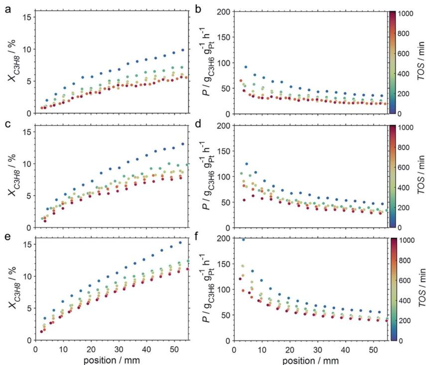
Fig. 8 Conversion profiles of propane, and productivity as a function of the catalyst bed length at various points in time during PDH over GaPt/SiO<sub>2</sub> SCALMS with an atomic ratio of Ga/Pt of 55 at (a and b) 450 °C, (c and d) 500 °C, and (e and f) 550 °C. Conditions of the experiment: 22 mL<sub>N</sub> min<sup>-1</sup> He; 3 mL<sub>N</sub> min<sup>-1</sup> C<sub>3</sub>H<sub>8</sub>; WHSV 4500 mL<sub>N</sub> g<sup>-1</sup> h<sup>-1</sup>.
