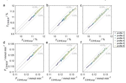
Fig. 6 Parity plots of the experimental and fitted (a–c) gas fractions and (d–f) molar flows of propane of the six profiles acquired at approx. 82, 259, 437, 614, 791, and 969 min time on stream during PDH over GaPt/SiO<sub>2</sub> SCALMS with an atomic ratio of Ga/Pt of 55 at (a and d) 450, (b and e) 500, and (c and f) 550 °C.
