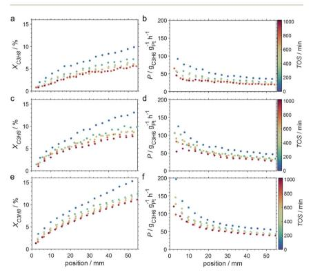
Fig. 8 Conversion profiles of propane, and productivity as a function of the catalyst bed length at various points in time during PDH over GaPt/SiO<sub>2</sub> SCALMS with an atomic ratio of Ga/Pt of 55 at (a and b) 450 °C, (c and d) 500 °C, and (e and f) 550 °C. Conditions of the experiment: 22  $\rm mL_N~min^{-1}~He;~3~mL_N~min^{-1}~C_3H_8;~WHSV~4500~mL_N~g^{-1}~h^{-1}.$
