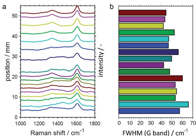
Fig. 10 (a) Spatially resolved Raman spectra of the catalyst bed after propane dehydrogenation over GaPt/Al<sub>2</sub>O<sub>3</sub> SCALMS with an atomic ratio of Ga/Pt of 86 with (b) the corresponding full width at half maximum (FWHM) of the G band of carbon at a Raman shift of 1605 cm<sup>-1</sup>. Conditions of the experiment: 500 °C; 22 mL<sub>N</sub> min<sup>-1</sup> He; 3 mL<sub>N</sub> min<sup>-1</sup> C<sub>3</sub>H<sub>8</sub>; WHSV 4500 mL<sub>N</sub> g<sup>-1</sup> h<sup>-1</sup>.
