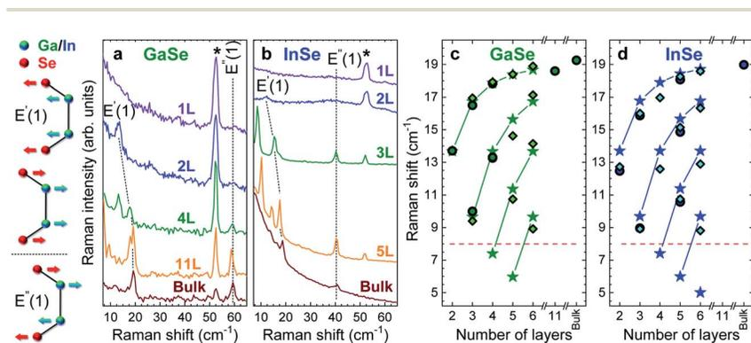
Fig. 5 Atomic displacements of phonon modes and unpolarized 514.5 nm low-frequency Raman spectra as a function of  $N$  for (a) GaSe and (b) InSe. Dashed lines are guides to the eye. (c and d)  $N$  dependence of C modes of (c) GaSe and (d) InSe. Circles and diamonds denote experimental results. Stars are DFT calculations. Dashed red horizontal lines represent the minimal Raman shift  $\sim 8$   $\text{cm}^{-1}$  detectable in our experiments.
