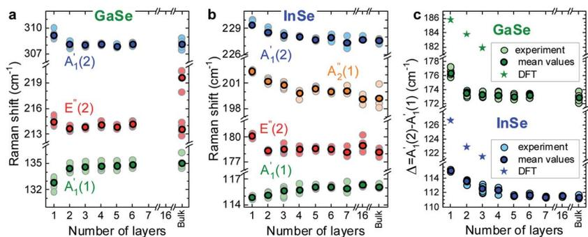
Fig. 4  $N$ -dependent Raman shifts for (a) GaSe and (b) InSe. (c)  $N$  dependence of  $\Delta = A_1'(2) - A_1'(1)$ . DFT calculations are indicated by star symbols. The dark color symbols correspond to mean values for the dataset shown in light colors measured at 633, 533, 514.5, 488 and 457 nm.
