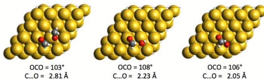
Figure 3. Structures of the three transition states associated with the A<sub>N</sub>2 of O, OH and CH<sub>3</sub>O onto CH<sub>2</sub>O.
