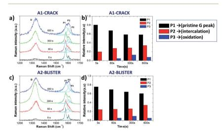
Fig. 3 Raman spectra acquired from certain areas of the HOPG surface during electrochemical oxidation in 0.5 M H<sub>2</sub>SO<sub>4</sub> electrolyte; (a and c) Raman spectra in the D and G band regions for the A1 and A2 areas; (b and d) Evolution with increasing time of Raman P1, P2 and P3 peaks for the A1 and A2 areas.
