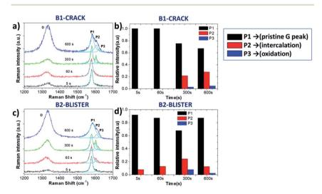
Fig. 5 Raman spectra acquired from certain areas of the HOPG surface during electrochemical oxidation in 0.5 M  $\text{Li}_2\text{SO}_4$  electrolyte; (a and c) Raman spectra in the D and G band regions for the B1 and B2 areas; (b and d) evolution with increasing time of Raman P1, P2 and P3 peaks for the B1 and B2 areas.
