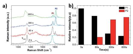
Fig. 8 (a) Raman spectra acquired from the HOPG surface during electrochemical oxidation in 1 M NaClO<sub>4</sub>/CH<sub>3</sub>CN electrolyte. (b) Evolution with increasing time of Raman P1 and P2 peaks.
