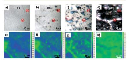
Fig. 4 (a-d) Optical images of the HOPG surface during electrochemical oxidation in 0.5 M  $\rm Li_2SO_4$  electrolyte and (e-h) the corresponding  $\rm I_D/I_G$  Raman mapping images.
