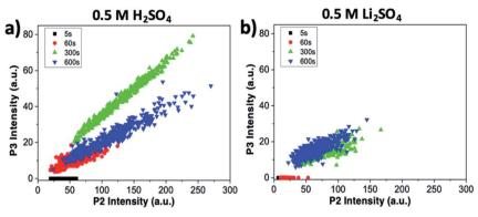
Fig. 6 Correlation between intercalation (P2) and oxidation of the sample (P3), obtained from Raman maps at different oxidation times. Graphs refer to (a) treatment in sulfuric acid and (b) treatment in lithium sulfate.
