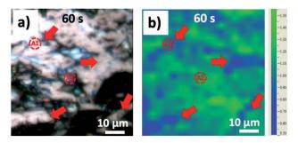
Fig. 2 (a) Optical image of HOPG surface and (b) the corresponding  $I_{\rm D}/I_{\rm G}$  Raman mapping image after 60 seconds' electrochemical oxidation in 0.5 M H<sub>2</sub>SO<sub>4</sub> electrolyte.
