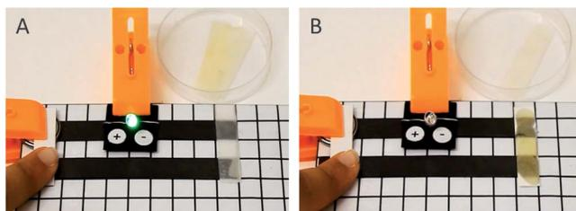
Fig. 7 Pictures of a circuit board assembled from a kit made for student experiments on electricity and electrochemistry. A piece of filter paper wetted with (A) an aqueous solution of NaCl ( $0.1 \text{ mol L}^{-1}$ ) and (B) cooking oil is placed between the conductive leads. A LED indicates the onset of electric current and it is lit on the left only.
