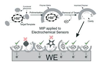
Fig. 4 Schematic representing MIPs applied to electrochemical sensor
