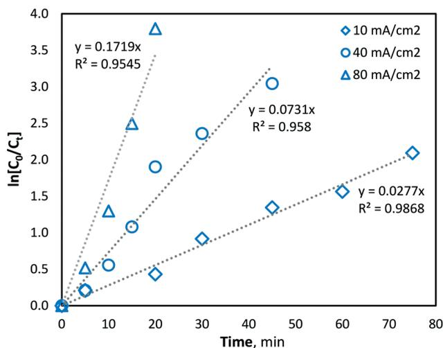
Fig. 4 Indirect quantification of hydroxyl radical formation (methanol degradation) with current densities of 10, 40 and 80  $\text{mA cm}^{-2}$  ( $\text{pH} = 7$ ,  $T = 21.0 \pm 0.8 \text{ }^\circ\text{C}$ ).
