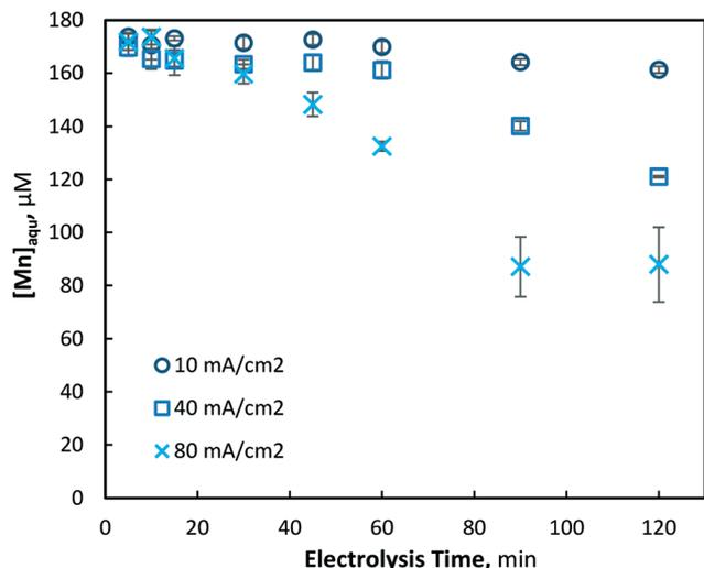
Fig. 2 Removal of aqueous manganese ( $\text{Mn}^{2+}$ ) with electrolysis time and current densities of 10, 40 and 80  $\text{mA cm}^{-2}$  ( $\text{pH} = 7$ ,  $[\text{Mn}^{2+}]_0 = 175 \mu\text{M}$ ,  $T = 21.0 \pm 0.8 \text{ }^\circ\text{C}$ ).
