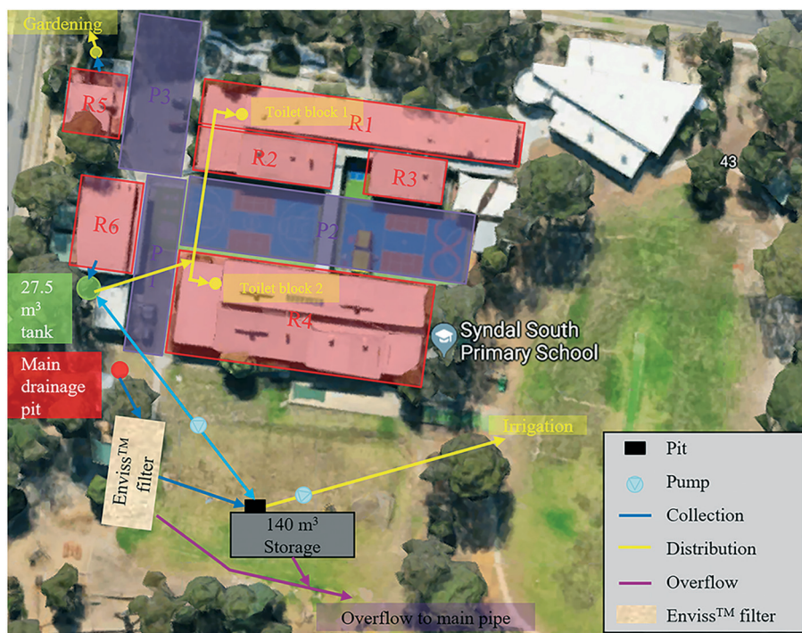
Fig. 1 South Syndal Primary School stormwater treatment and harvesting set-up.
