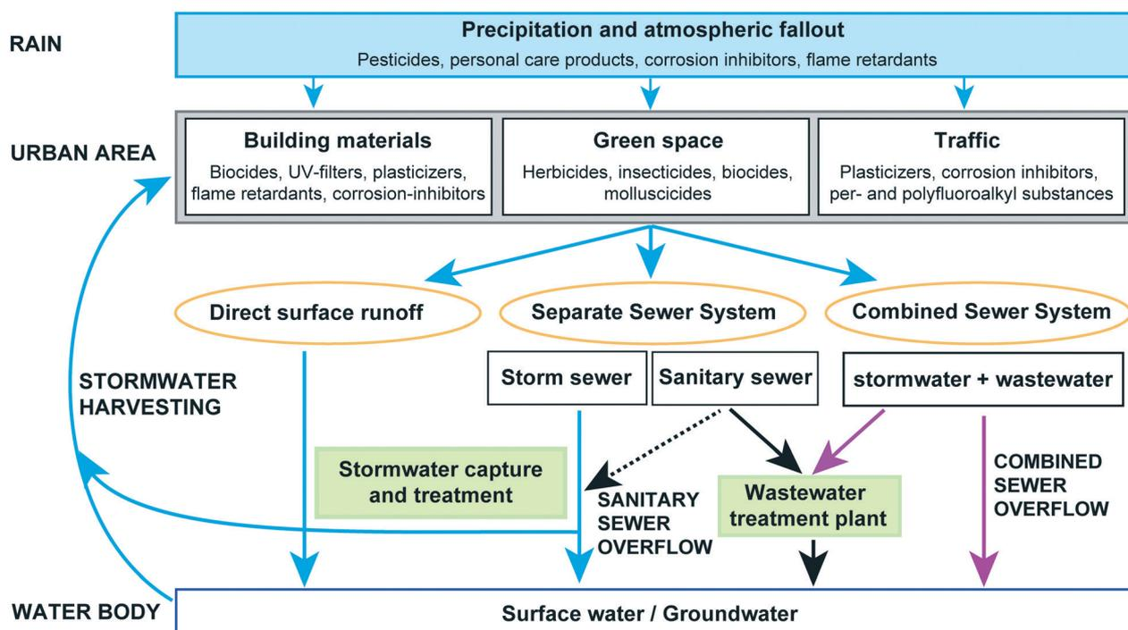
Fig. 1 Sources of hydrophilic trace organic contaminants (hyphil-TrOCs) in urban stormwater and input paths of stormwater- and wastewater-derived hyphil-TrOCs into receiving waters. Stormwater harvesting for the urban water supply requires stormwater capture and treatment technologies.
