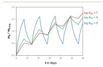
Fig. 4 Illustrative simulations of uptake curves of three hypothetical chemicals in response to fluctuating air concentrations  $C_G$ . Fluctuations in the amount of a chemical sequestered in a PAS increase with increasing volatility, i.e. decreasing log  $K_{SG}$ .
