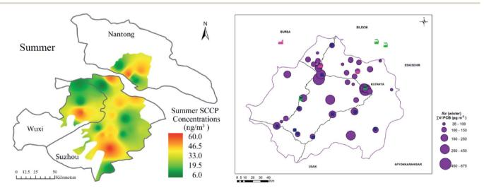
Fig. 10 Two examples of how spatial variability in air concentrations as determined by PAS networks has been displayed, either using interpolation<sup>360</sup> (left) or not<sup>363</sup> (right). Reproduced from ref. 360 and 363 with permission from Elsevier, Copyright 2017 and 2020.
