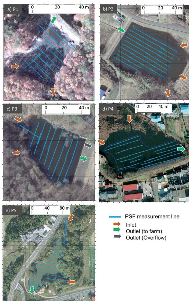
Fig. 3 PSF measuring lines in each studied pond. Also shown are the inlets and outlets of each pond. Satellite images © ArC GIS, ESRI, Co, Ltd., USA.
