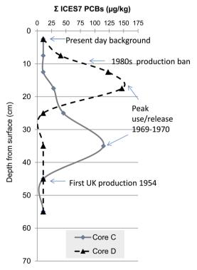
Fig. 7 Vertical changes in polychlorinated biphenyls (PCB) concentration in four sediment cores from Chiswick Ait, River Thames.
