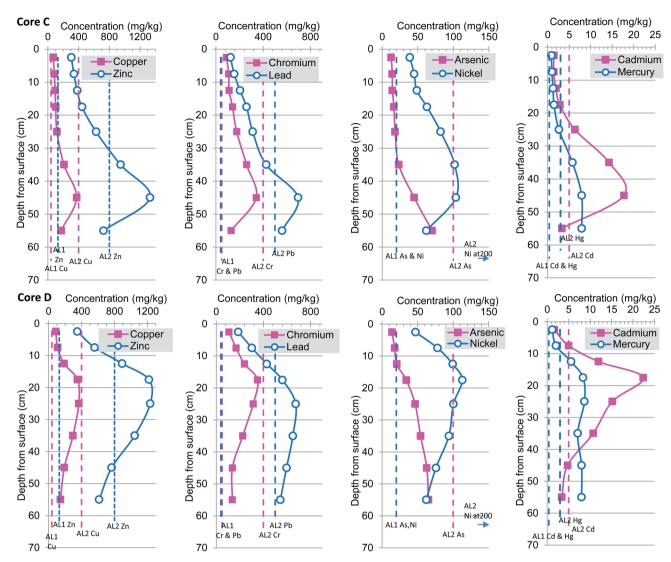
Heavy metal concentrations profiles for cores C and D. Dashed vertical lines represent non-statutory sediment quality guidelines
