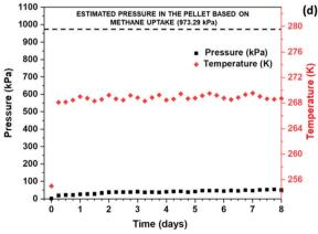
Fig. 6 (a) Diameter, (b) length and (c) weight of the synthesized mixed methane–DIOX hydrate pellet. (d) Demonstration of the stable storage of the mixed methane–DIOX hydrate pellet at atmospheric pressure and moderate temperature of 268.15 K.
