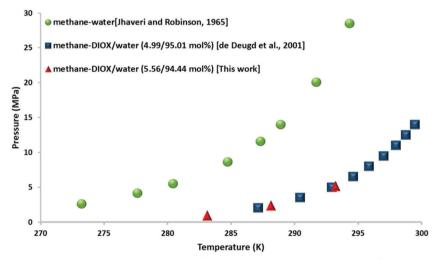
Fig. 1 Three-phase (H-Lw-V) equilibrium points for methane-water<sup>29</sup> and methane-DIOX/water systems<sup>27</sup> together with the experimental data obtained in the present study for the methane-DIOX/water system containing a stoichiometric concentration of DIOX (5.56 mol%).
