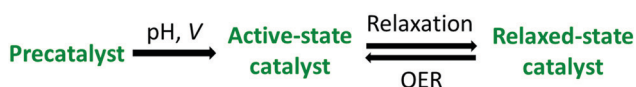
Scheme 1 Transformation of a precatalyst to the active catalyst. The reversible step on the right side shows the dynamic behavior of the catalyst, which can be assessed by in situ investigations.
