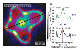
Fig. 2 (a) Static PL distribution of the MAPbl<sub>3</sub> grain. The position of the excitation laser spot is marked with the red cross. An increased PL is detected at the grain boundaries, most likely due to enhanced outcoupling of wave-guided PL. (b) and (c) show the intensity distributions corresponding to the green and black line-profiles in (a), with local maxima at the position of the excitation as well as the grain boundaries.
