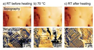
Fig. 6 AFM topography (top row) and corresponding lateral PFM phase (a) before (at 26  $^{\circ}$ C), (b) during (at 70  $^{\circ}$ C) and (c) after (at 27  $^{\circ}$ C) the heating experiment over the cubic-tetragonal phase transition at 54  $^{\circ}$ C, visualizing a change in the domain pattern following the heating cycle.
