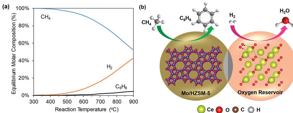
Fig. 11 (a) Equilibrium product composition of CH<sub>4</sub> DHA as a function of reaction temperature. (b) A potential configuration of methane CL-DHA process (the air regeneration step is not shown).<sup>240</sup>
