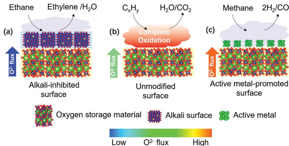
Fig. 9 Schematic illustration of surface modifications of redox catalysts to improve product selectivity by changing the relative rates of surface oxygen removal and bulk O<sup>2-</sup> flux. The arrows in the three cases (a–c) correspond to the O<sup>2-</sup> fluxes and the colors correspond to the relative intensity of the O<sup>2-</sup> fluxes.
