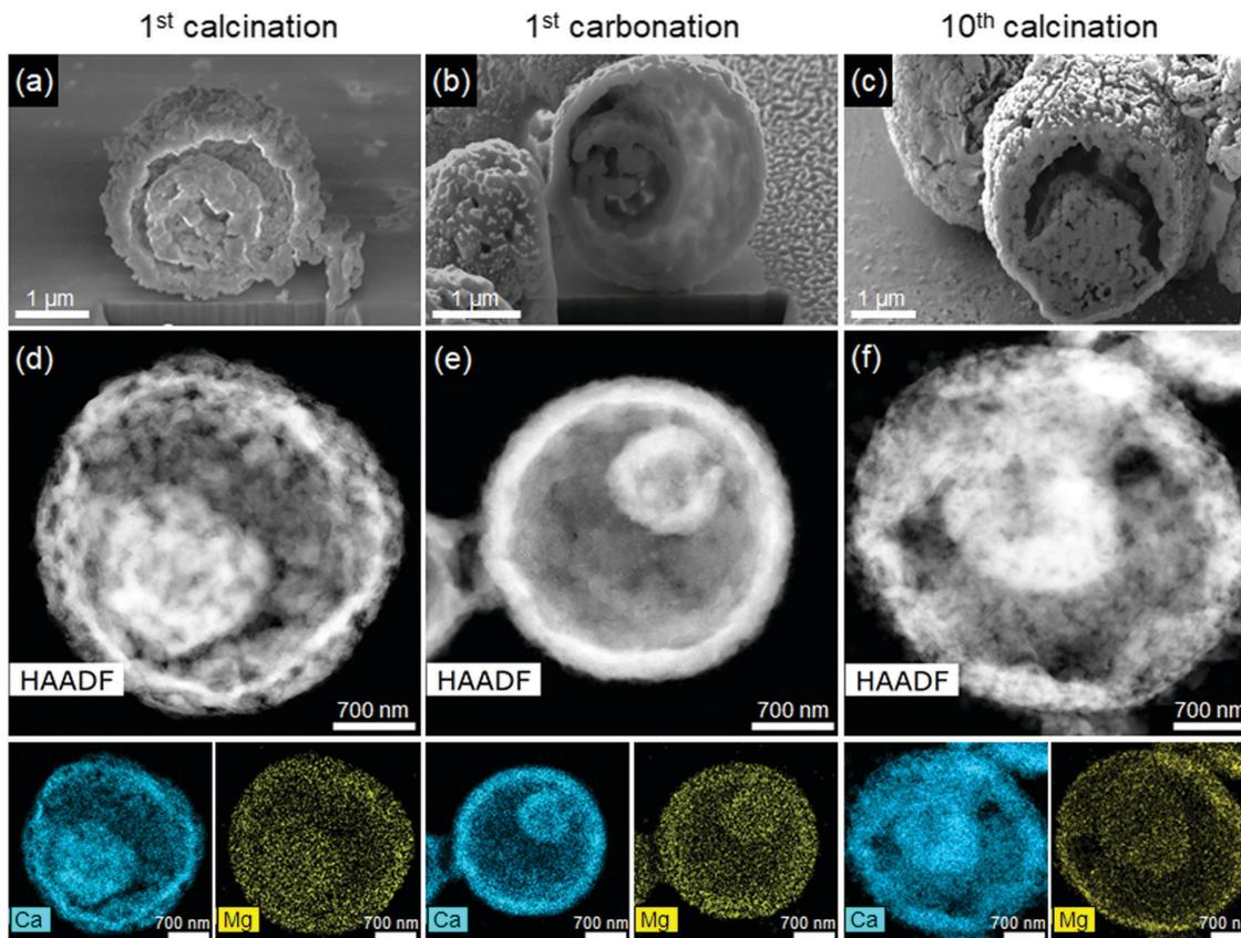
Fig. 15 Morphological changes during cyclic operation of a Ca–Mg mixed oxide-based sorbent. (a–c) SEM images of FIB cross-sections. (d–f) HAADF-STEM images with EDX maps of Ca and Mg at different stages of CO<sub>2</sub> capture/regeneration cycles. Scale bars: 1 μm for (a–c) and 700 nm for (d–f).<sup>451</sup>
