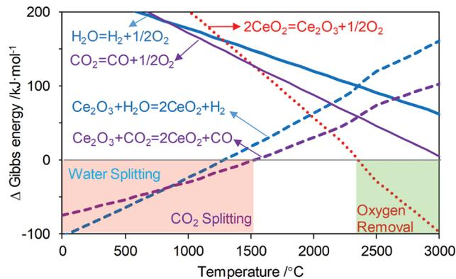
Fig. 4 Ellingham diagram of thermal and chemical looping water and CO<sub>2</sub> splitting. Light green and red regions represent thermodynamically spontaneous ( $K \geq 1$ ) reduction and oxidation reactions, respectively. In practice, a reaction would occur when  $K < 1$ .
