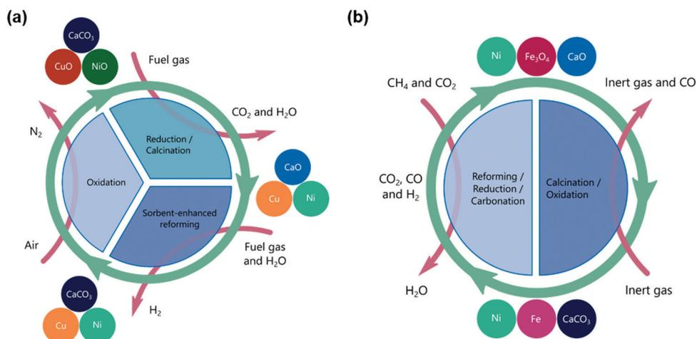
Fig. 14 (a) Reaction scheme with three reactors where  $\text{CuO}$ -based chemical looping combustion is integrated into the SE-SMR process. (b) Reaction scheme of the super-dry reforming of methane with two reactors, in which the reforming catalyst (Ni) is spatially separated from the oxygen carrier ( $\text{Fe}_3\text{O}_4$ ) and the  $\text{CO}_2$  sorbent.
