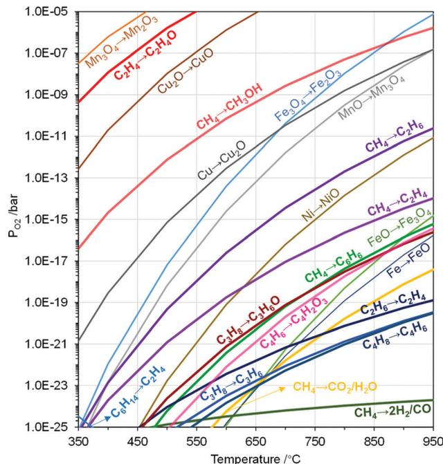
Fig. 8 Modified Ellingham diagram of metal oxide redox and POx reactions.  $\text{MeO}_x \rightarrow \text{MeO}_y$  and hydrocarbons POx reactions correspond to the  $P_{\text{O}_2}$  when  $\Delta G = 0$ . Reactions in pathways of  $\text{MeO}_x \rightarrow \text{MeO}_y$  and hydrocarbons POx are given in Table 2.
