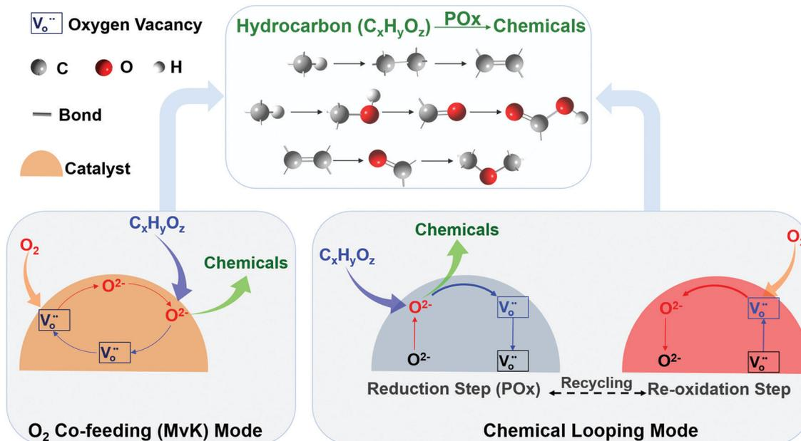
Fig. 16 Comparison of  $O_2$  co-feeding (MvK) and chemical looping modes for partial oxidations and their applications on conversions of hydrocarbon to chemicals (transformation between alkane, alkene, alcohol, aldehyde, ketone, acid, and aromatics).
