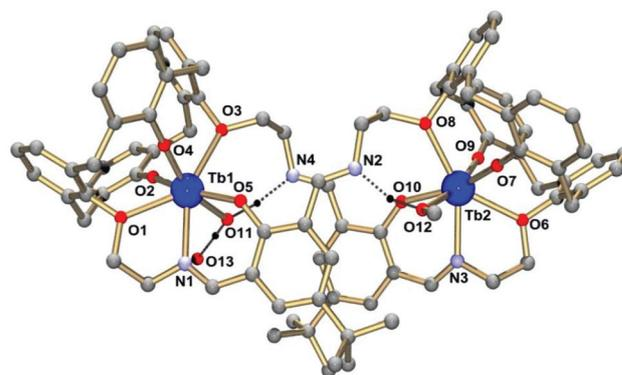
Fig. 5 Single-crystal X-ray diffraction structure of the dinuclear  $[\text{Tb}_2(\text{L}^2)(\text{MeOH})(\text{H}_2\text{O})]$  complex in crystals of  $3 \cdot (\text{H}_2\text{O})_x$ ,  $x \sim 10$  (ball-and-stick representation). Dashed lines refer to intramolecular hydrogen bonding interactions ( $\text{O11} \cdots \text{N4} = 2.75 \text{ \AA}$ ,  $\text{O11} \cdots \text{O13} = 2.78 \text{ \AA}$ ,  $\text{O12} \cdots \text{N2} = 2.62 \text{ \AA}$ ).
