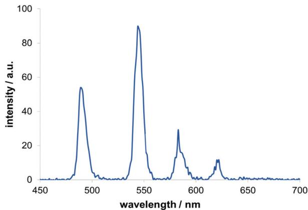
Fig. 9 Emission spectrum of a  $5 \times 10^{-5}$  M solution of complex **3** in H<sub>2</sub>O/DMSO (95/5 v/v, HEPES-buffer,  $1 \times 10^{-2}$  M concentration, pH 7.4). Excitation wavelength  $\lambda_{\text{ex}}$  292 nm.
