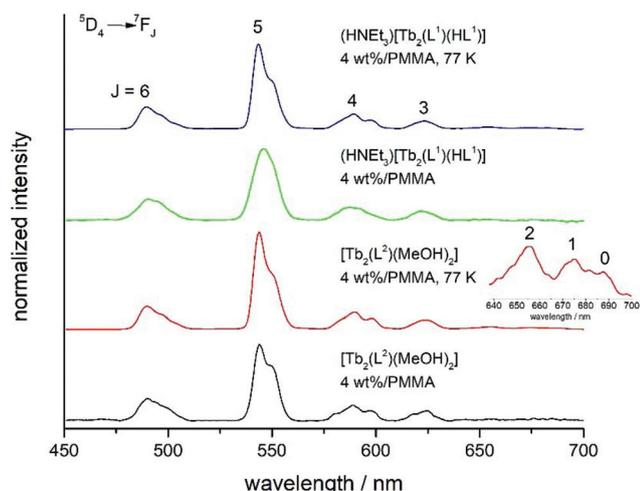
**Fig. 8** Photoluminescence spectra of  $[\text{HNEt}_3][\text{Tb}_2(\text{HL}^1)(\text{L}^1)]$  and  $[\text{Tb}_2(\text{L}^2)(\text{MeOH})_2]$  (**3**) immobilized in a PMMA thin film (4 wt% **3**, thickness  $\sim 0.2$  mm) at 77 K and 298 K. The excitation wavelength is 361 nm. The spectra are normalized with respect to the  $^5\text{D}_4 \rightarrow ^7\text{F}_6$  transition.
