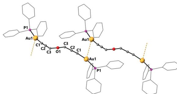
**Fig. 5** Molecular structure of complex 7 determined by single crystal X-ray diffraction showing intermolecular aurophilic interactions. Selected bond lengths [Å] and angles [°]: Au(1)–C(1) 2.060(9), Au(1)–C(1B) 1.951(9), Au(1)–P(1) 2.2733(12), Au(1)–Au(1)#1 3.2907(4), C(1)–C(2) 1.205(2), C(2)–C(3) 1.439(2), C(1)–Au(1)–P(1) 168.0(7), C(1)–C(2)–C(3) 177.6(18). In complex 7 the oxygen atom is disordered, only distances to the main component are included.
