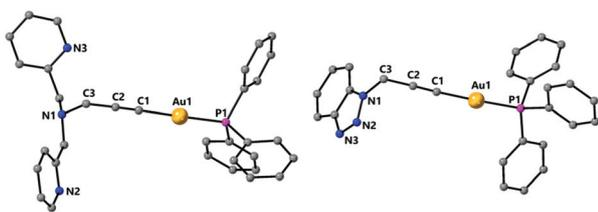
**Fig. 2** Molecular structures of complexes 2 and 4 determined by single crystal X-ray diffraction. Selected bond lengths [Å] and angles [°]: 2: Au(1)–C(1) 2.024(5), Au(1)–P(1) 2.2711(13), C(1)–C(2) 1.173(7), C(2)–C(3) 1.487(8), C(1)–Au(1)–P(1) 178.95(15), C(1)–C(2)–C(3) 176.6(6); 4: Au(1)–C(1) 1.997(3), Au(1)–P(1) 2.2772(8), C(1)–C(2) 1.198(4), C(2)–C(3) 1.468(4), C(1)–Au(1)–P(1) 175.31(8), C(1)–C(2)–C(3) 178.7(3).
