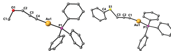
Fig. 4 Molecular structures of complexes 5 and 8 determined by single crystal X-ray diffraction. Selected bond lengths [Å] and angles [°]: 5: Au(1)–C(4) 2.005(5), Au(1)–P(1) 2.2870(12), O(1)–C(1) 1.393(7), O(1)–C(2) 1.416(6), C(2)–C(3) 1.489(7), C(3)–C(4) 1.205(7), C(4)–Au(1)–P(1) 178.38(15), C(4)–C(3)–C(2) 174.4(5); 8: Au(1)–C(1) 1.994(3), Au(1)–P(1) 2.2766(7), S(1)–C(4) 1.763(3), S(1)–C(3) 1.818(4), C(1)–C(2) 1.206(4), C(2)–C(3) 1.467(4), C(1)–Au(1)–P(1) 173.51(9), C(1)–C(2)–C(3) 175.1(3).
