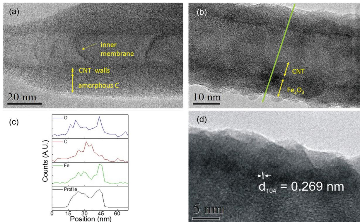
Fig. 3 High resolution TEM analysis of (a) pristine utCNTs. CNT walls, inner membranes and the amorphous C layer are indicated by arrows. (b) 6 nm  $\text{Fe}_2\text{O}_3$ @wpCNTs; (c) elemental line profile of O, C and Fe acquired along the green line marked in (b). (d) High resolution TEM of the  $\text{Fe}_2\text{O}_3$  coating on wpCNTs revealing an interplanar spacing of  $d \sim 0.269$  nm for iron oxide.
