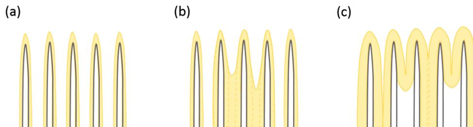
Fig. 2 Illustration of different ALD coatings of  $\text{Fe}_2\text{O}_3$  on the CNT surface: (a) conformal coating; (b) partial conformal coating and partial CNT aggregation; (c) thicker and non-conformal coating on CNTs.
