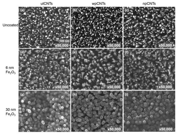
Fig. 1 SEM micrographs of pristine, 6 nm and 30 nm ALD Fe<sub>2</sub>O<sub>3</sub> coated untreated (utCNTs), water plasma treated (wpCNTs) and nitrogen plasma treated carbon nanotubes (npCNTs). The bar scale corresponds to 100 nm in all the images.
