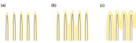
Fig. 2 Illustration of different ALD coatings of  $Fe_2O_3$  on the CNT surface: (a) conformal coating; (b) partial conformal coating and partial CNT aggregation; (c) thicker and non-conformal coating on CNTs.
