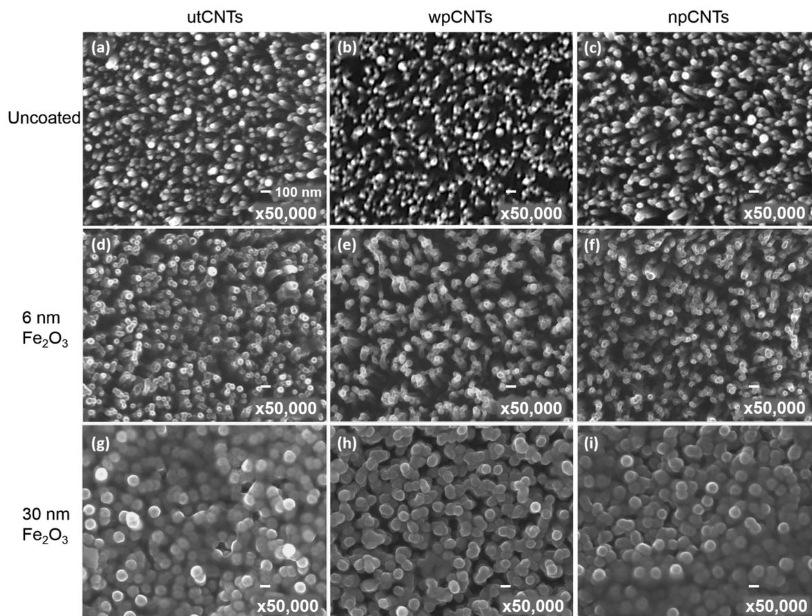
**Fig. 1** SEM micrographs of pristine, 6 nm and 30 nm ALD Fe<sub>2</sub>O<sub>3</sub> coated untreated (utCNTs), water plasma treated (wpCNTs) and nitrogen plasma treated carbon nanotubes (npCNTs). The bar scale corresponds to 100 nm in all the images.
