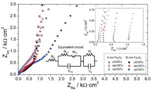
Fig. 9 Nyquist plot of different CNT samples covered with 6 and 30 nm iron oxide by ALD. The inset shows the intersection with the real axis in the high-frequency region and the modified Randles equivalent circuit used to fit the data
