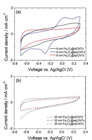
Fig. 6 Areal capacitance of carbon nanotubes with and without plasma treatment, covered with 6 and 30 nm thickness ALD-iron oxide at a  $50 \text{ mV s}^{-1}$  scan rate.
