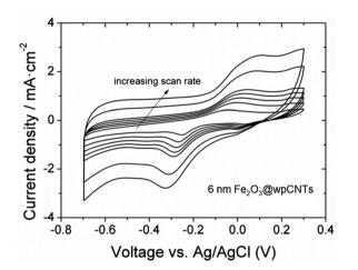
Fig. 7 Cyclic voltammograms of 6 nm  $\rm Fe_2O_3@wpCNTs$  at scan rates from 10 to 150 mV s $^{-1}$ .
