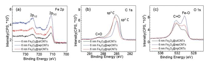
Fig. 5 (a) High-resolution Fe 2p spectra; (b) C 1s spectra and (c) O 1s spectra of 6 nm Fe<sub>2</sub>O<sub>3</sub>@CNTs.
