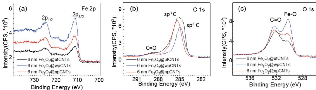
Fig. 5 (a) High-resolution Fe 2p spectra; (b) C 1s spectra and (c) O 1s spectra of 6 nm Fe<sub>2</sub>O<sub>3</sub>@CNTs.
