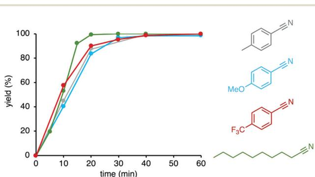
**Fig. 3** Time-dependent profiles for the catalytic oxidation towards nitrile with complex **5** under ammonia gas (6 mL) and molecular oxygen. General conditions: Amine substrate (0.2 mmol), [Ru] (0.01 mmol, 5 mol%), 1,2-dichlorobenzene (2 mL), 150 °C. Conversions were determined by <sup>1</sup>H NMR integration (1,3,5-trimethoxybenzene as internal standard) and are averaged over 2 runs. Isolated yields between 52% (4-Me-benzonitrile) and 86% (4-MeO-benzonitrile).
