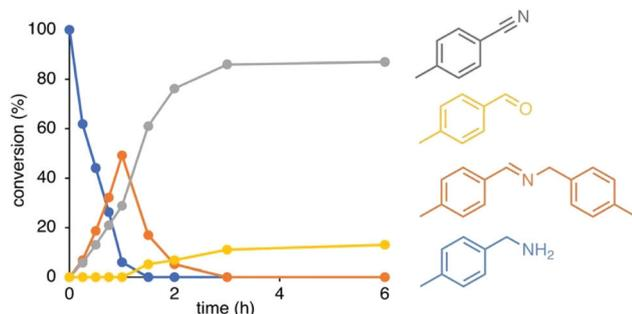
Fig. 2 Time-dependent conversion profile for the catalytic oxidation of 4-methylbenzylamine with complex **4b**. General conditions: 4-Methylbenzylamine (0.2 mmol), [Ru] (0.01 mmol, 5 mol%), 1,2-dichlorobenzene (2 mL), 150 °C. Conversions were determined by <sup>1</sup>H NMR integration (1,3,5-trimethoxybenzene as internal standard) and are averaged over 2 runs.
