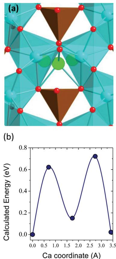
Fig. 2 (a) View of the Ca diffusion pathway in  $\text{Ca}_4\text{Fe}_9\text{O}_{17}$ , showing the tetrahedral site at the transition state. (b) Calculated energy barrier. Color code: Ca sites in blue, diffusing Ca in green, Fe in brown, O in red.
