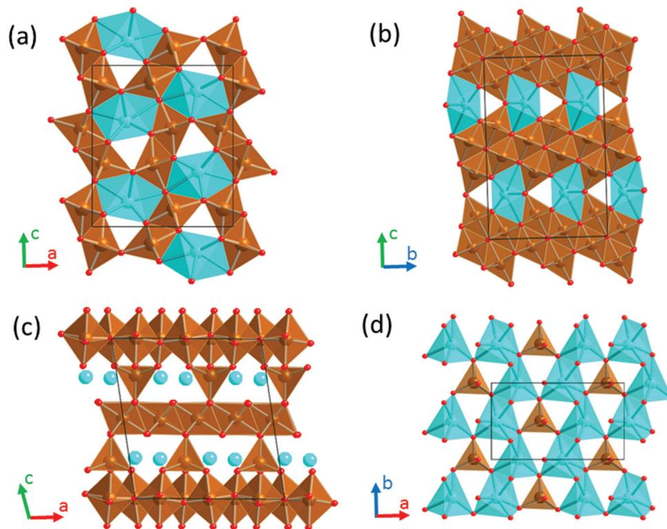
**Fig. 1** Crystal structures of  $\text{CaFe}_{2+n}\text{O}_{4+n}$  oxides. (a)  $n = 0$ ,  $\text{CaFe}_2\text{O}_4$  (b)  $n = 2$ ,  $\text{CaFe}_4\text{O}_6$  (c)  $n = 1/4$ ,  $\text{Ca}_4\text{Fe}_9\text{O}_{17}$  showing the  $[\text{CaO}_6]$ - $[\text{FeO}_4]$  plane in (d). Color code: Ca in blue, Fe in brown and O in red.
