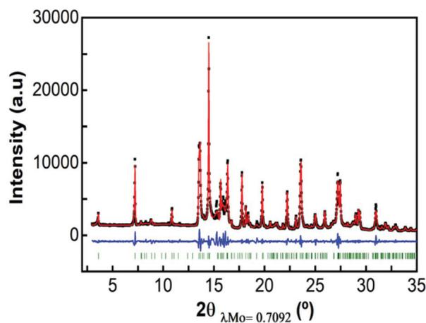
Fig. 3 Pattern matching of  $\text{Ca}_4\text{Fe}_9\text{O}_{17}$  in the monoclinic system, space group  $C2$ .
