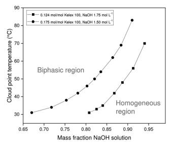
Fig. 3 Variation of cloud point temperature of [EhEhT<sub>23</sub>]<sub>2</sub>[SO<sub>4</sub>] and sodium hydroxide solutions with the composition of the mixture.
