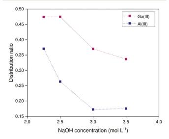
Fig. 9 Distribution ratio of gallium as a function of the NaOH concentration in the stripping liquor for loaded 0.124 mol mol $^{-1}$  Kelex® 100 in [EhEhT $_{23}$ ] $_4$ [SO $_4$ ], extracted from 200 ppm solutions containing 1.700 mol L $^{-1}$  sodium carbonate in 1:1 phase ratio (organic to aqueous). Temperature: 22 °C.
