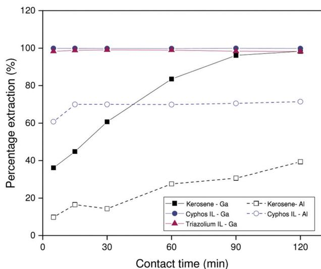
Fig. 5 Percentage extraction as a function of time for 200 ppm solutions extracted from 1.700 mol L<sup>-1</sup> sodium carbonate by 5 vol% Kelex® 100 in [EhEhT<sub>23</sub>][SO<sub>4</sub>], 5 vol% Kelex® 100 in [C101]<sub>2</sub>[SO<sub>4</sub>] and 5 vol% Kelex® 100 in kerosene modified with 10 vol% 1-decanol. Phase ratio: 1 : 1 organic to aqueous. The HLLC procedure was followed for [EhEhT<sub>23</sub>][SO<sub>4</sub>].
