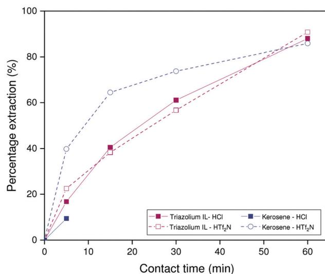
**Fig. 12** Percentage extraction as a function of time for extractions performed in 1 : 1 phase ratio by organic phases saturated with 1 mol L<sup>-1</sup> HCl or hydrogen bistriflimide. The composition of the organic phase was 5 vol% Kelex 100 in [HHT<sub>12</sub>][Tf<sub>2</sub>N] or kerosene (modified with 10 vol% 1-decanol) and the aqueous phase was 2 mol L<sup>-1</sup> NaOH containing 873 mmol L<sup>-1</sup> NaAl(OH)<sub>4</sub> and 150 ppm Ga. Temperature: 22 °C.
