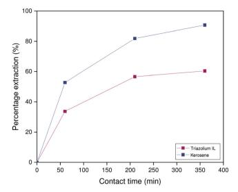
Fig. 11 Percentage extraction as a function of time for extractions performed in 1:1 phase ratio by 5 vol% Kelex 100 in  $[HHT_{12}][Tf_2N]$  or kerosene (modified with 10 vol% 1-decanol) from 2 mol  $L^{-1}$  NaOH containing 873 mmol  $L^{-1}$  NaAl(OH)<sub>4</sub> and 150 ppm Ga. Temperature: 22 °C.
