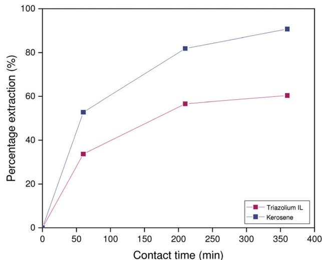
**Fig. 11** Percentage extraction as a function of time for extractions performed in 1 : 1 phase ratio by 5 vol% Kelex 100 in [HHT<sub>12</sub>][Tf<sub>2</sub>N] or kerosene (modified with 10 vol% 1-decanol) from 2 mol L<sup>-1</sup> NaOH containing 873 mmol L<sup>-1</sup> NaAl(OH)<sub>4</sub> and 150 ppm Ga. Temperature: 22 °C.
