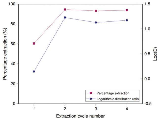
**Fig. 10** Percentage extraction and logarithmic distribution ratio of gallium over several extraction/stripping cycles. Extraction was performed in 1 : 1 phase ratio by 5 vol% Kelex 100 in [HHT<sub>12</sub>][Tf<sub>2</sub>N] (modified with 10 vol% 1-decanol) from 2 mol L<sup>-1</sup> NaOH containing 873 mmol L<sup>-1</sup> NaAl(OH)<sub>4</sub> and 150 ppm Ga. Stripping was performed with 1 mol L<sup>-1</sup> HCl. Temperature: 22 °C.
