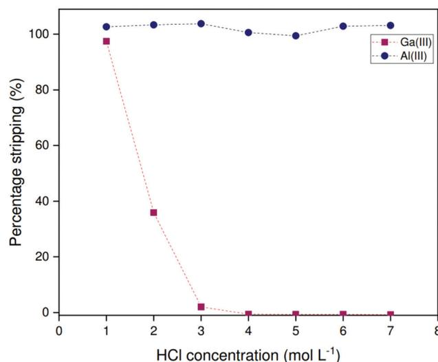
**Fig. 8** Percentage stripping of gallium and aluminum as a function of the HCl concentration in the stripping liquor for loaded 5 vol% Kelex® 100 in [HHT<sub>12</sub>][Tf<sub>2</sub>N] modified with 10 vol% 1-decanol, extracted from 200 ppm solutions containing 2,000 mol L<sup>-1</sup> sodium hydroxide in 1 : 1 phase ratio (organic to aqueous). Temperature: 22 °C.
