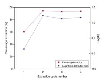
**Fig. 10** Percentage extraction and logarithmic distribution ratio of gallium over several extraction/stripping cycles. Extraction was performed in 1:1 phase ratio by 5 vol% Kelex 100 in [HHT<sub>12</sub>][Tf<sub>2</sub>N] (modified with 10 vol% 1-decanol) from 2 mol L<sup>-1</sup> NaOH containing 873 mmol L<sup>-1</sup> NaAl(OH)<sub>4</sub> and 150 ppm Ga. Stripping was performed with 1 mol L<sup>-1</sup> HCl. Temperature: 22 °C.
