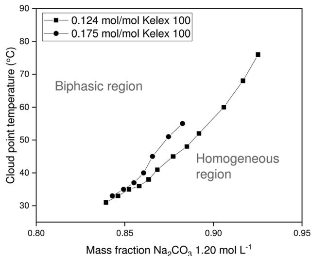
Fig. 4 Variation of cloud point temperature of [EhEhT<sub>23</sub>]<sub>2</sub>[SO<sub>4</sub>] and sodium carbonate solutions with the composition of the mixture.
