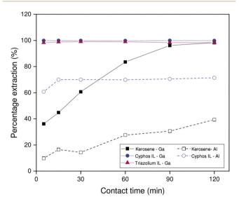
Fig. 5 Percentage extraction as a function of time for 200 ppm solutions extracted from 1.700 mol L<sup>-1</sup> sodium carbonate by 5 vol% Kelex® 100 in [EhEhT<sub>23</sub>]<sub>2</sub>[SO<sub>4</sub>], 5 vol% Kelex® 100 in [C101]<sub>2</sub>[SO<sub>4</sub>] and 5 vol% Kelex® 100 in kerosene modified with 10 vol% 1-decanol. Phase ratio: 1:1 organic to aqueous. The HLLE procedure was followed for  $[EhEhT_{23}]_2[SO_4].$
