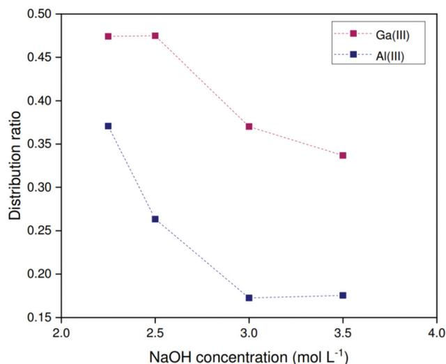
**Fig. 9** Distribution ratio of gallium as a function of the NaOH concentration in the stripping liquor for loaded  $0.124 \text{ mol mol}^{-1}$  Kelex® 100 in  $[\text{EhEt}_{23}]_4[\text{SO}_4]$ , extracted from 200 ppm solutions containing  $1.700 \text{ mol L}^{-1}$  sodium carbonate in 1 : 1 phase ratio (organic to aqueous). Temperature:  $22^\circ\text{C}$ .
