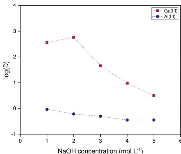
Fig. 7 Variation of the logarithmic distribution ratios of gallium and aluminum with the sodium hydroxide concentration of the feed for 200 ppm solutions extracted by 5 vol% Kelex® 100 in [HHT<sub>12</sub>][Tf<sub>2</sub>N] modified with 10 vol% 1-decanol. Phase ratio: 1 : 2 (organic to aqueous). Temperature: 25 °C.
