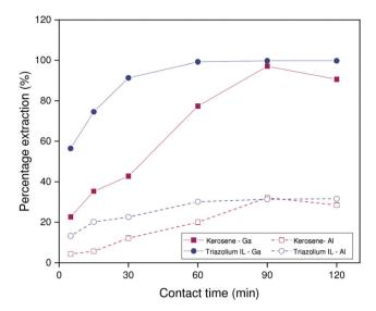
Fig. 6 Percentage extraction as a function of time for 200 ppm solutions extracted from 1.700 mol L<sup>-1</sup> sodium carbonate by 5 vol% Kelex® 100 in [HHT<sub>12</sub>][Tf<sub>2</sub>N] modified with 10 vol% 1-decanol, and 5 vol% Kelex® 100 in kerosene modified with 10 vol% 1-decanol. Phase ratio: 1:1 organic to aqueous. Temperature: 22 °C.
