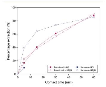
Fig. 12 Percentage extraction as a function of time for extractions performed in 1:1 phase ratio by organic phases saturated with 1 mol L $^{-1}$  HCl or hydrogen bistriflimide. The composition of the organic phase was 5 vol% Kelex 100 in [HHT $_{12}$ ][Tf $_2$ N] or kerosene (modified with 10 vol% 1-decanol) and the aqueous phase was 2 mol L $^{-1}$  NaOH containing 873 mmol L $^{-1}$  NaAl(OH) $_4$  and 150 ppm Ga. Temperature: 22 °C.
