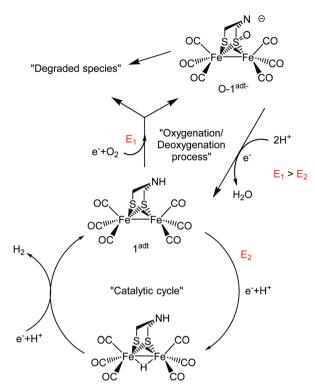
Scheme 1 Summary of the mechanism for oxygenation/deoxygenation processes and the catalytic cycle for  $H_2$  evolution catalyzed by  $\mathbf{1}^{adt}$ . The red character, E is the reduction potential.
