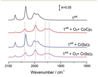
Fig. 3 The formation of a new species, O-1<sup>adt-</sup> by mixing 1<sup>adt</sup>, O<sub>2</sub> and reductants,  $CoCp_2$  or  $Cr(bz)_2$ . The complex  $\mathbf{1}^{adt}$  (0.36 mM) was first mixed with 4 eq. of CoCp<sub>2</sub> or 2 eq. of Cr(bz)<sub>2</sub> and then 4 eq. of O<sub>2</sub> from O<sub>2</sub>-saturated DCM solution was added.
